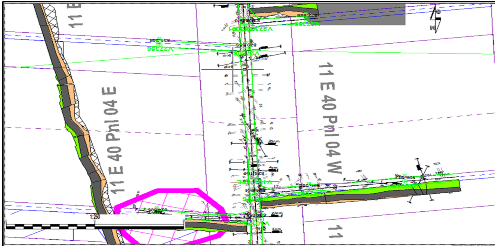
Fig 11: Typical underground mapping presented on MineCad software showing undulating UG2, minor faults, infill joints and deteriorated ground condition in a stoping area affected hydrothermal alteration (Lonmin Saffy Shaft database).
