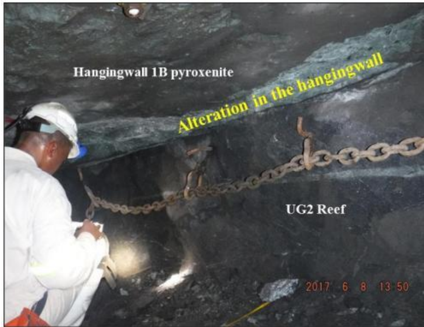
Fig 17 (a): Typical east of Saffy Shaft stope panel photo, showing the hydrothermal alteration above the UG2 reef horizon (Hartzenberg, 2019).
