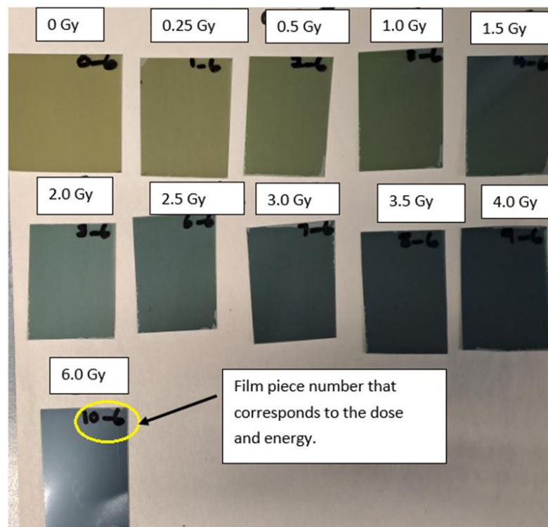
Figure 4. 24: Gafchromic EBT3 film calibration pieces irradiated to doses in the range 0 - 6 Gy using a 6 MV photon beam.
