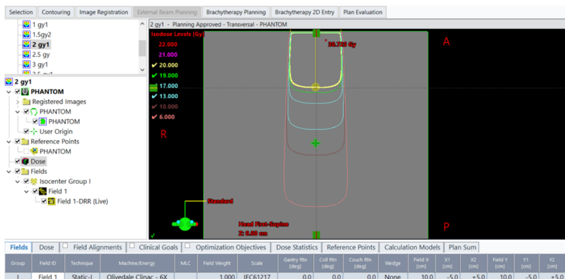
Figure 4. 17: Treatment plan dose distribution of a 6 MV photon beam of 2 Gy prescription dose normalized at isocentre (yellow isodose line) from the Varian Eclipse treatment planning system (Eclipse treatment planning system (TPS) (Varian Medical Systems, Palo Alto, CA)).
