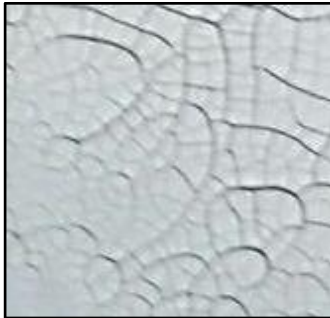
Figure 6-5: An image showing the cracked \text{TiO}_2 surface after exposing it air for 10 min.
