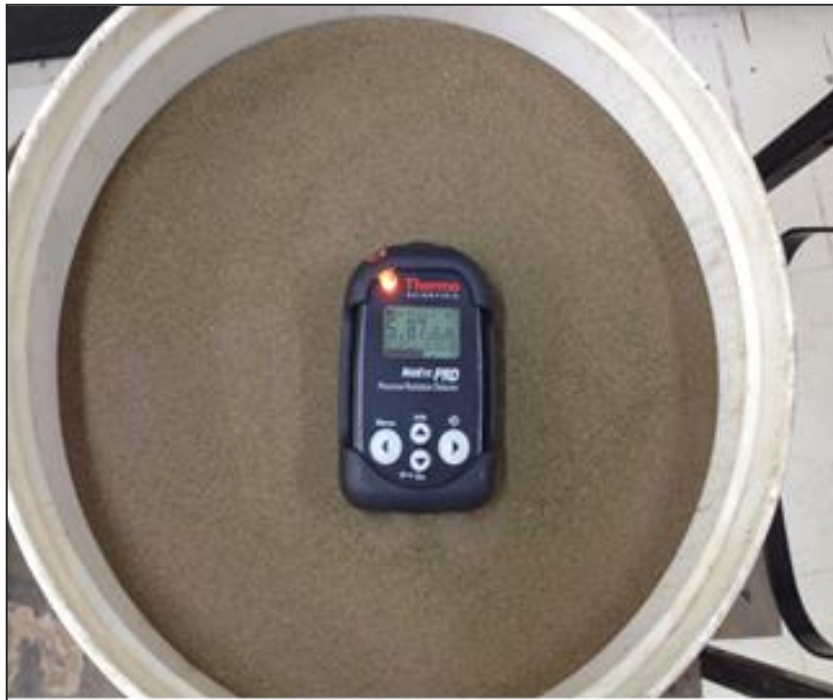
Figure 6: An image showing the 50kg bucket of the research sample, and the recorded radioactive reading of 5.87microsieverts per hour
