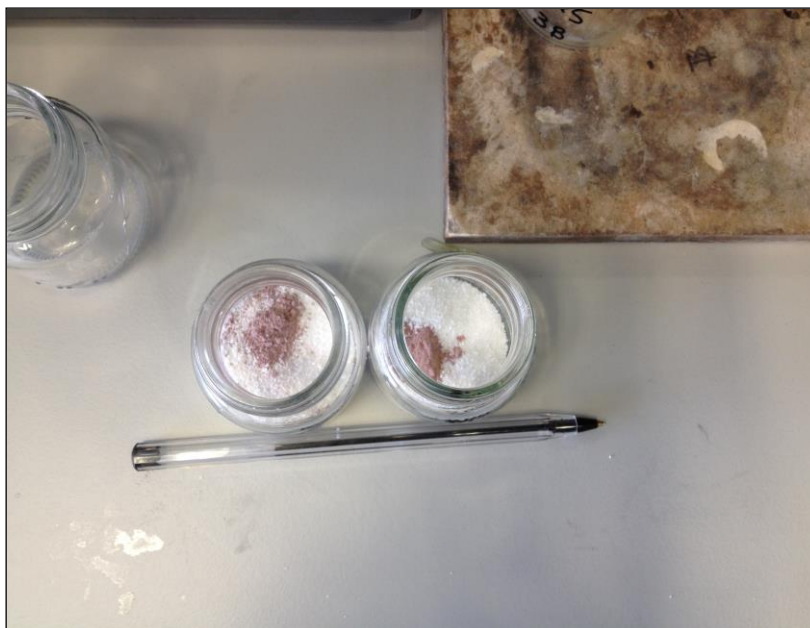
Figure 26: A photograph showing the sample mixture before alkali fusion.
