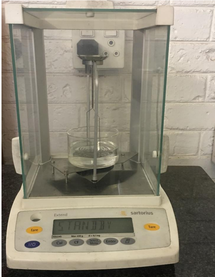
Figure 3.1: Macrograph of the densimeter used to measure the density of the investigated samples.
