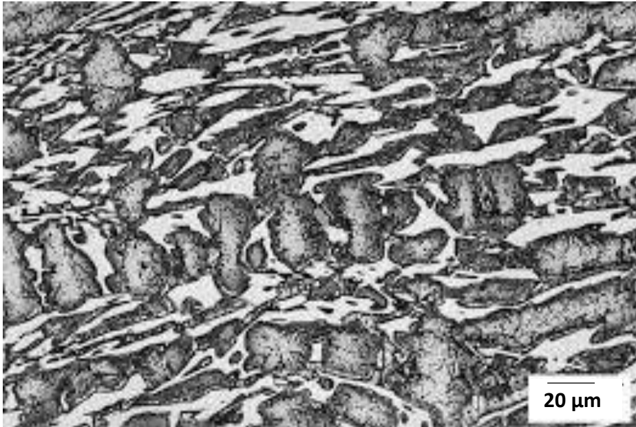
Figure 2.15: Optical micrograph showing microstructure of white cast iron ( Filipovic et al., 2012 ).
