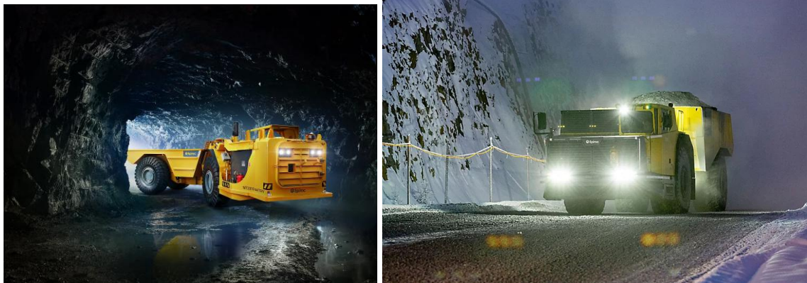
Figure 4 42-tonne payload capacity truck
