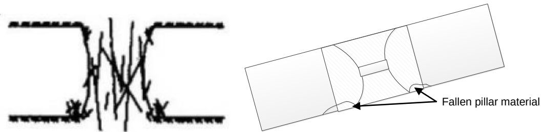
Figure 2.10 Failed pillar with internal shear fractures (Brady & Brown, 2005)
