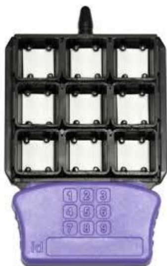
Figure 2.2 Randox biochip (nine, 9x9 mm wells) (Randox Laboratories Limited, 2021)
