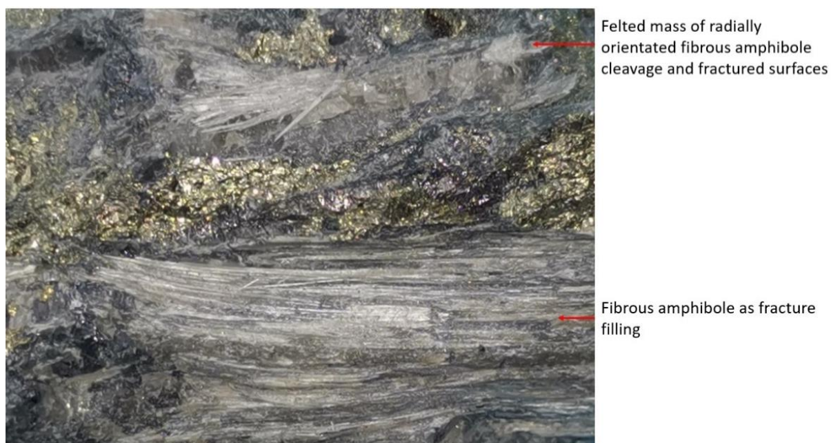
Figure 7.10: Textures observed in fibrous amphiboles, sulphides, and magnetite within the siderite host rock.
