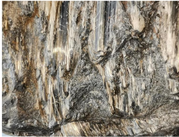
Figure 6.52: (Sample 18) Amosite seam having a waste cone without any amosite fibres
