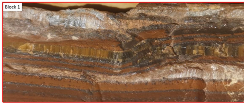
Figure 6.29: (sample 12) Complex dislocation structures between magnetite and bedding parallel fibrous quartz veins. Greyish blue slip fibre riebeckite at upper left part of the image.
