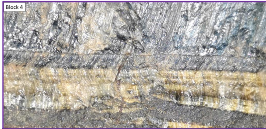
Figure 6.32: (sample 12) Dislocation structures formed between magnetite layers and marginal fibrous quartz.
