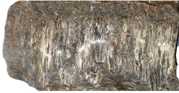
Figure 6.51: (Sample 18) Amosite asbestos rock sample; notice the wavy, uneven, and unclear bounding surfaces due to overgrowth of grunerite needles.
