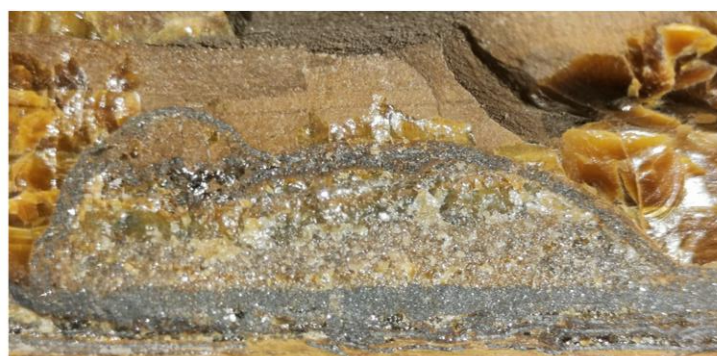
Figure 6.37: (sample 13) Highly unusual cone structure formed by large, coarse, multi-coloured, and interlocking quartz crystals. The cone shape is outlined by dark-grey magnetite laminae of varying thickness.
