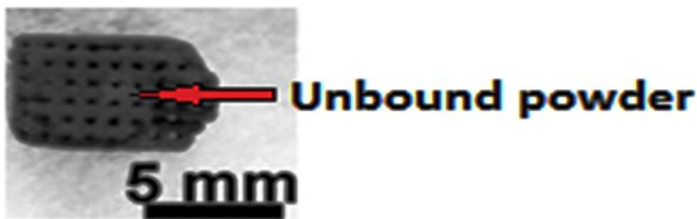
Figure 2.5: Photograph of prototype sample part of the 3D printed Fe–30Mn scaffold powder after sintering (Chou et al. , 2013).
