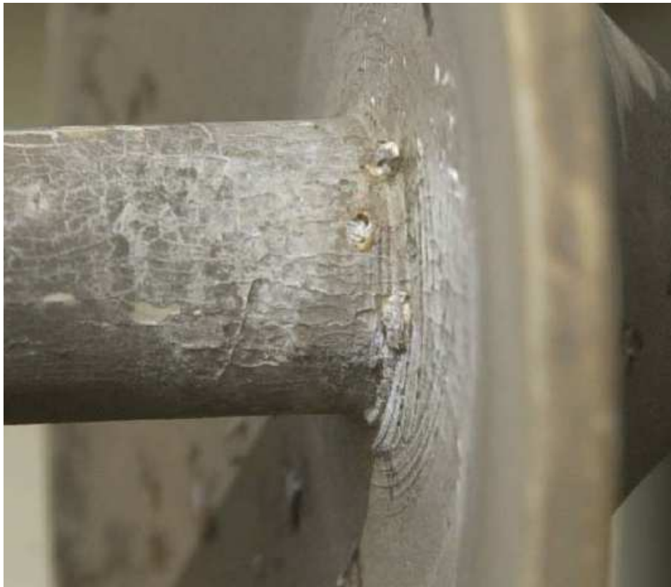
Figure 4.11: Visible puncture damage along the sheath of the test insulator, used with permission [35]
