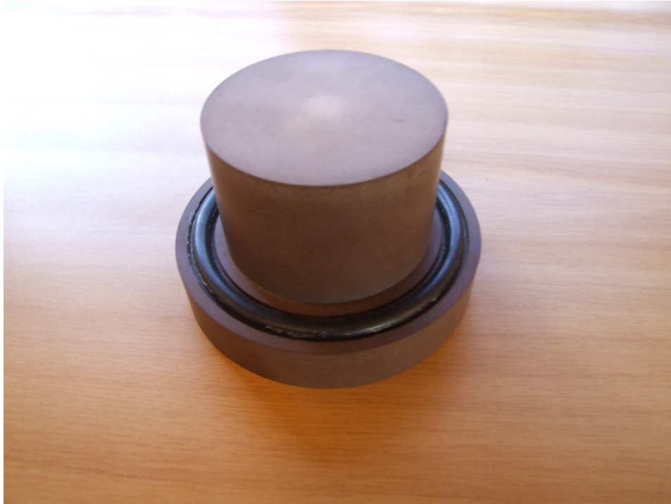
Figure 5.8: Designed and manufactured epoxy resin plug
