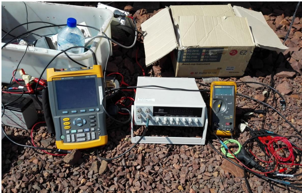
Figure 66: Photograph showing the experiment setup for AC measurements at the experiment location during the wagon measurements.
