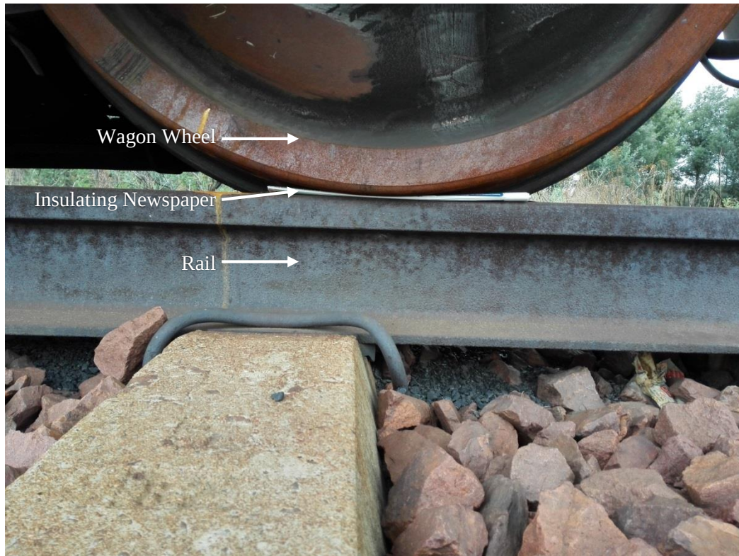
Figure 72: Photograph showing the paper isolation between the wagon wheels and rail during the wagon measurements.
