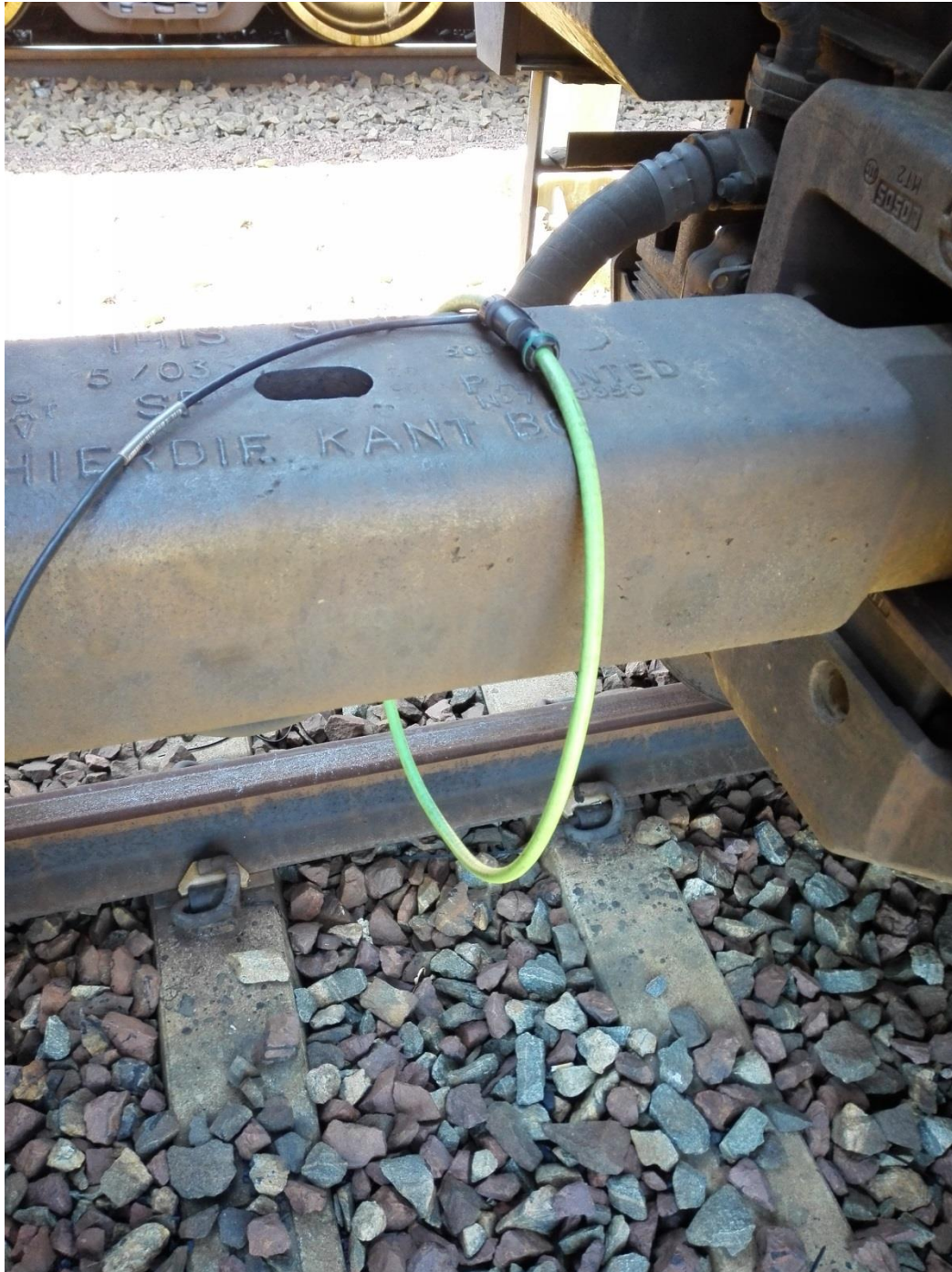
Figure 98: Photograph showing placement of the current clamp around the draw bar of one Transnet Freight Rail's coal wagon sets.
