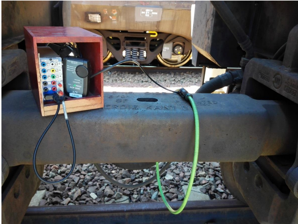
Figure 99: Photograph showing placement of the connection from the current clamp to the optic transmitter on one Transnet Freight Rail's coal wagon sets.
