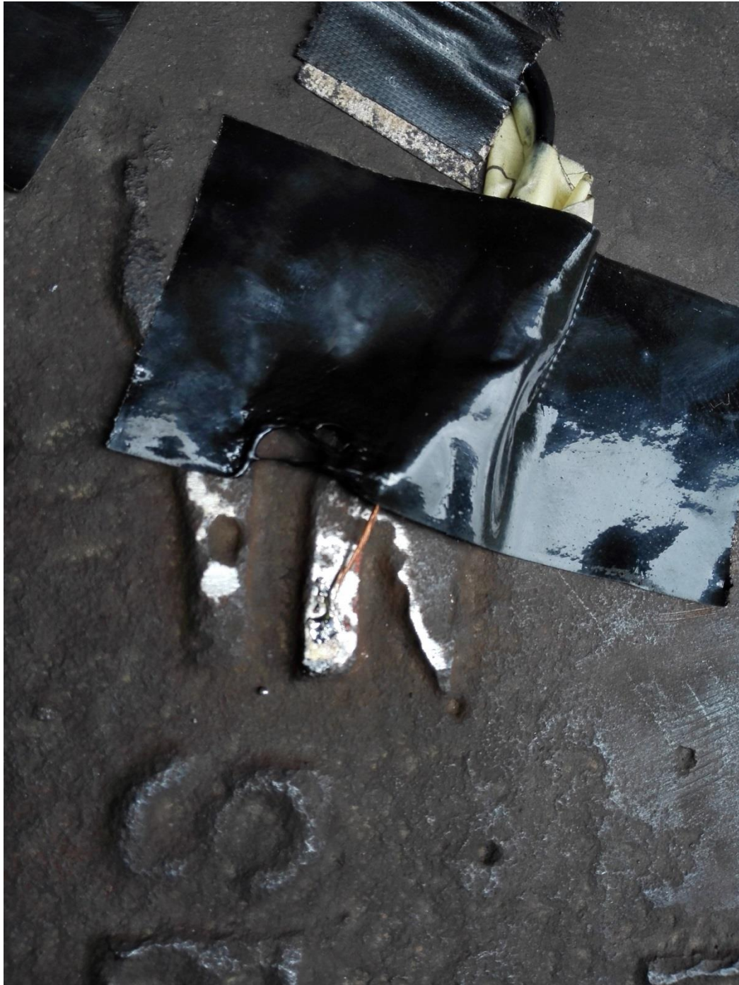
Figure 74: Photograph showing the solder connections between conductors and the nodes of the wagon during the wagon measurements.
