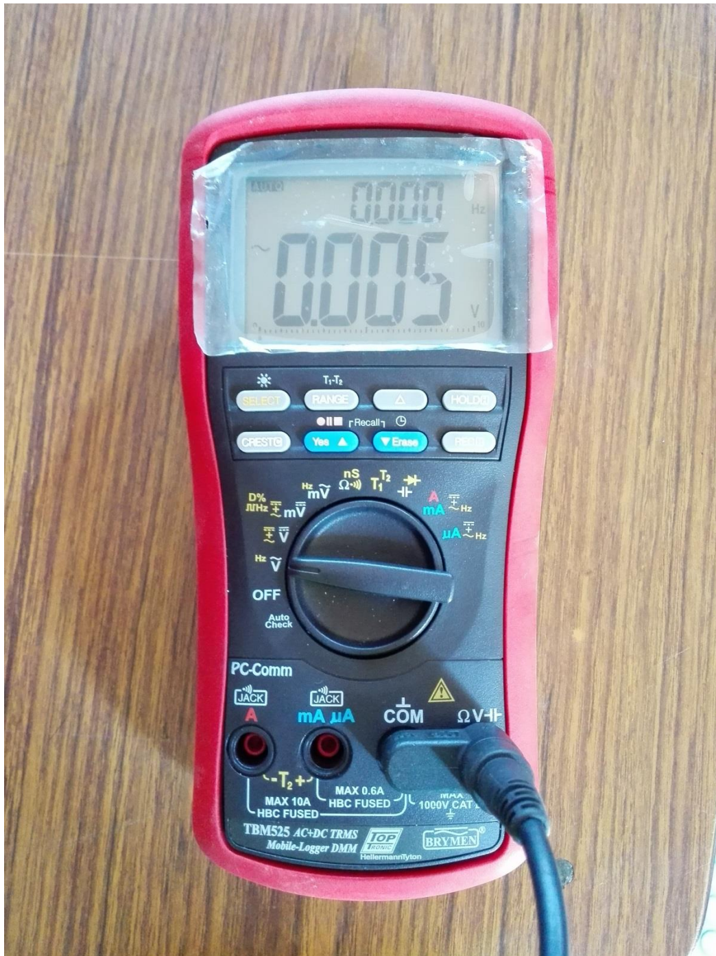
Figure 100: Photograph showing the remote logger used to measure wagon currents at significant distance from the Transnet Freight Rail test coach.
