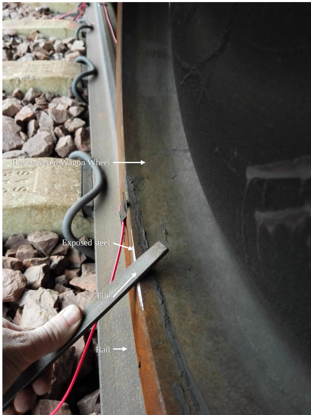
Figure 73: Photograph showing the filing of surfaces to which electrical contacts were made during the wagon measurements.
