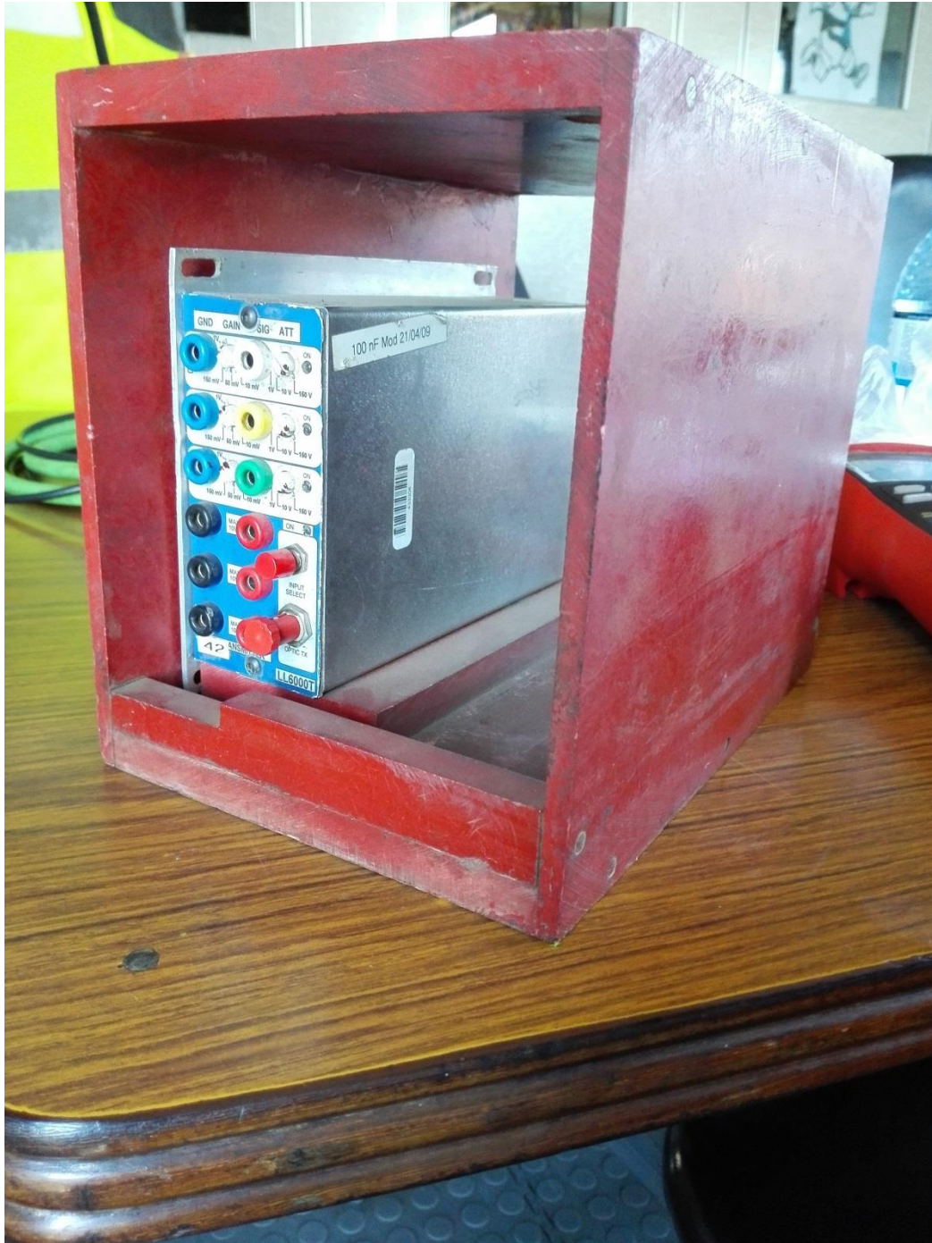
Figure 96: Photograph showing the front of the fibre optic transmitter on one of Transnet Freight Rail's test coaches.
