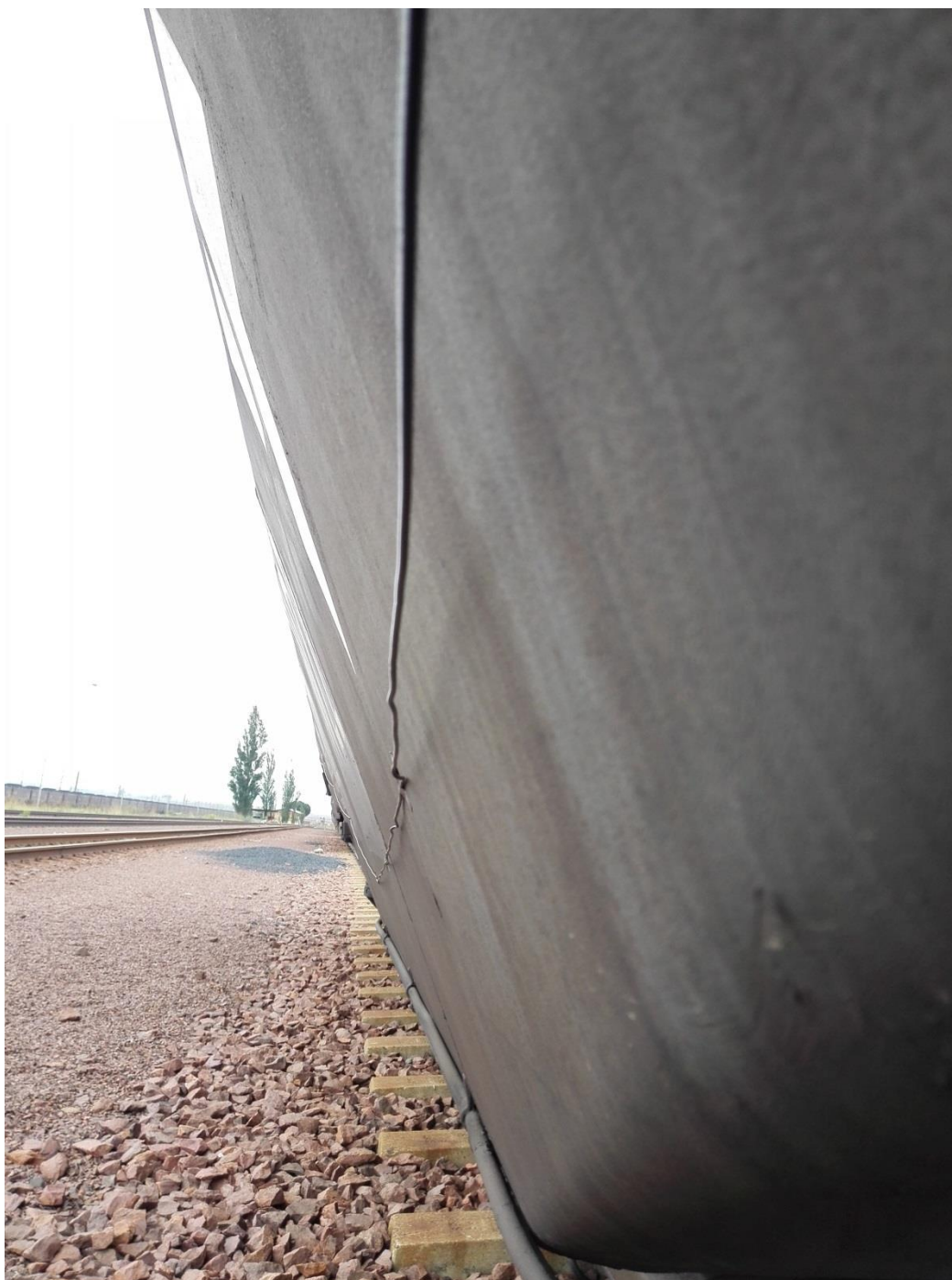
Figure 75: Photograph showing the return conductive wire in close proximity to the wagon body to avoid creating loop areas and inductances during the wagon measurements.
