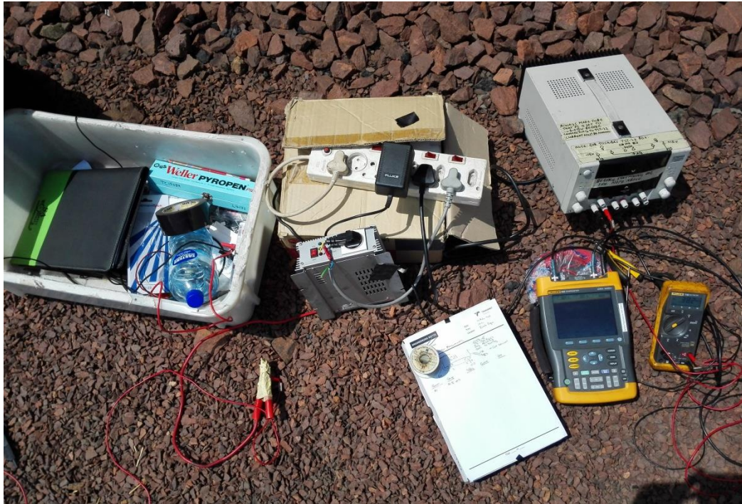
Figure 65: Photograph showing the experiment setup for DC measurements at the experiment location during the wagon measurements.
