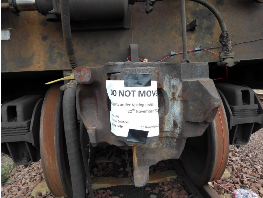
Figure 67: Photograph showing the warning notice not to couple to or move the wagon set which was under testing during the wagon measurements.
