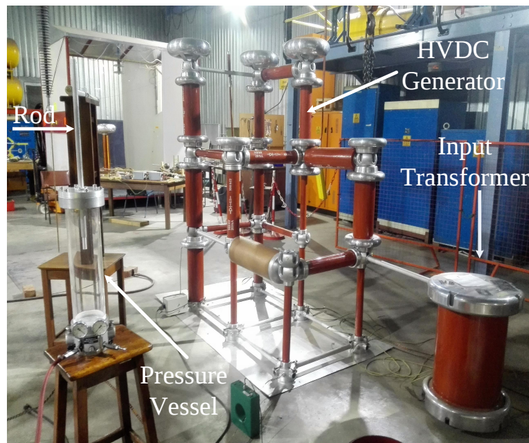
FIGURE 4.3: Pressure vessel test set-up in the HV lab at Wits University
