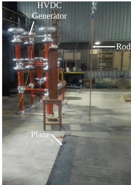
FIGURE 4.1: Open air test set-up in the HV lab at Wits University
