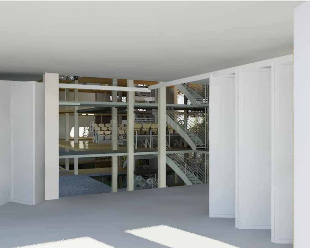
Figure 79: Sliding/stackaway partition details- The stack away and sliding partitions reside within the cavity walls, they are located within the parasites as well as along the main structural volume of the innovation centre space, these walls allow the flexibility of public space in the building to transition between market space, exhibitions and lecture venues(Author, 2022)
