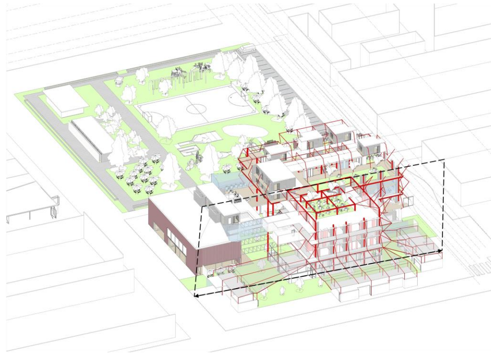
Figure 122: 3D Section and Axonometric illustrating column structural grid to show tectonic nature of structure in defining, the exhibition, lecture venues and market space(Author,2022)
