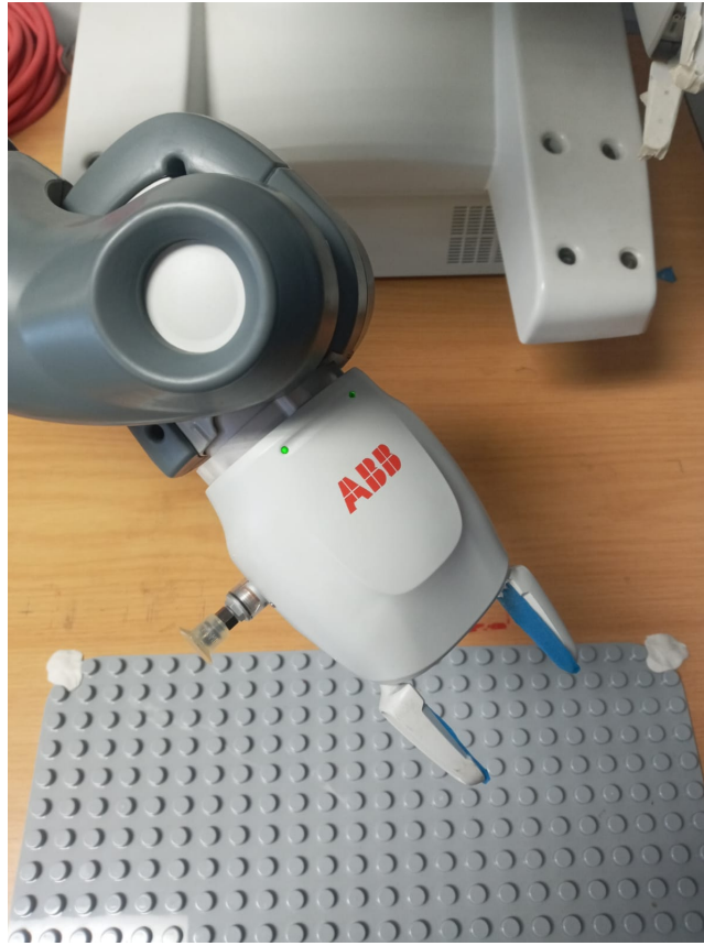
Figure 3.3: An illustration showing YuMi robot's pincer grippers.
