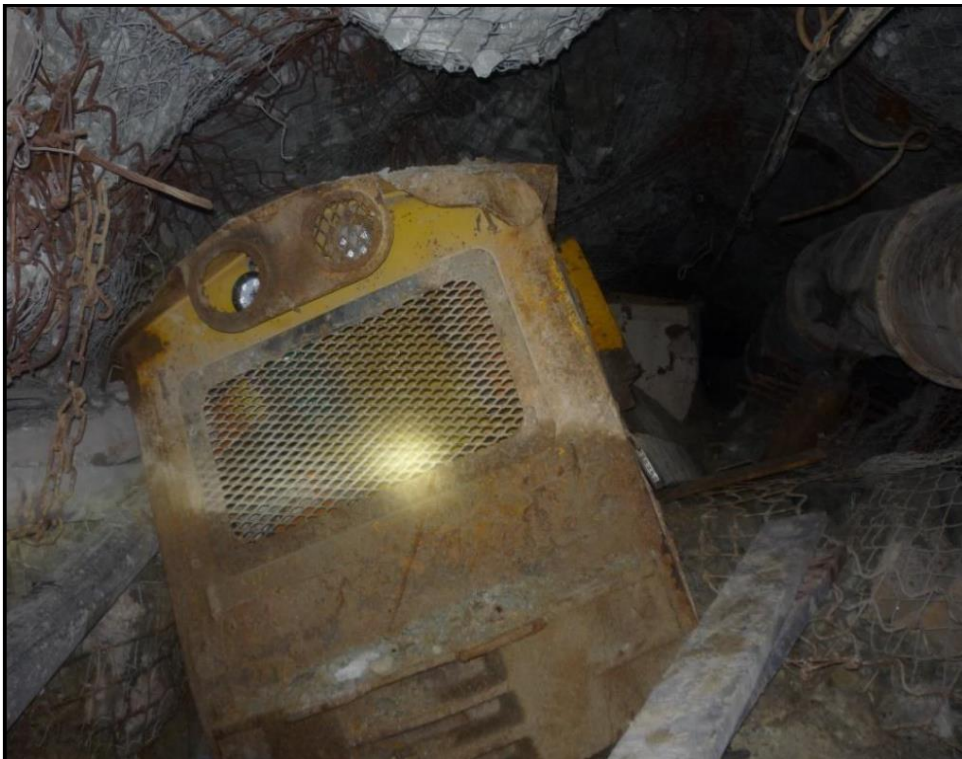
Figure 5.16: Footwall heave lifting a 5 ton locomotive above the grade line position (Tshepo Rabele, 2014).
