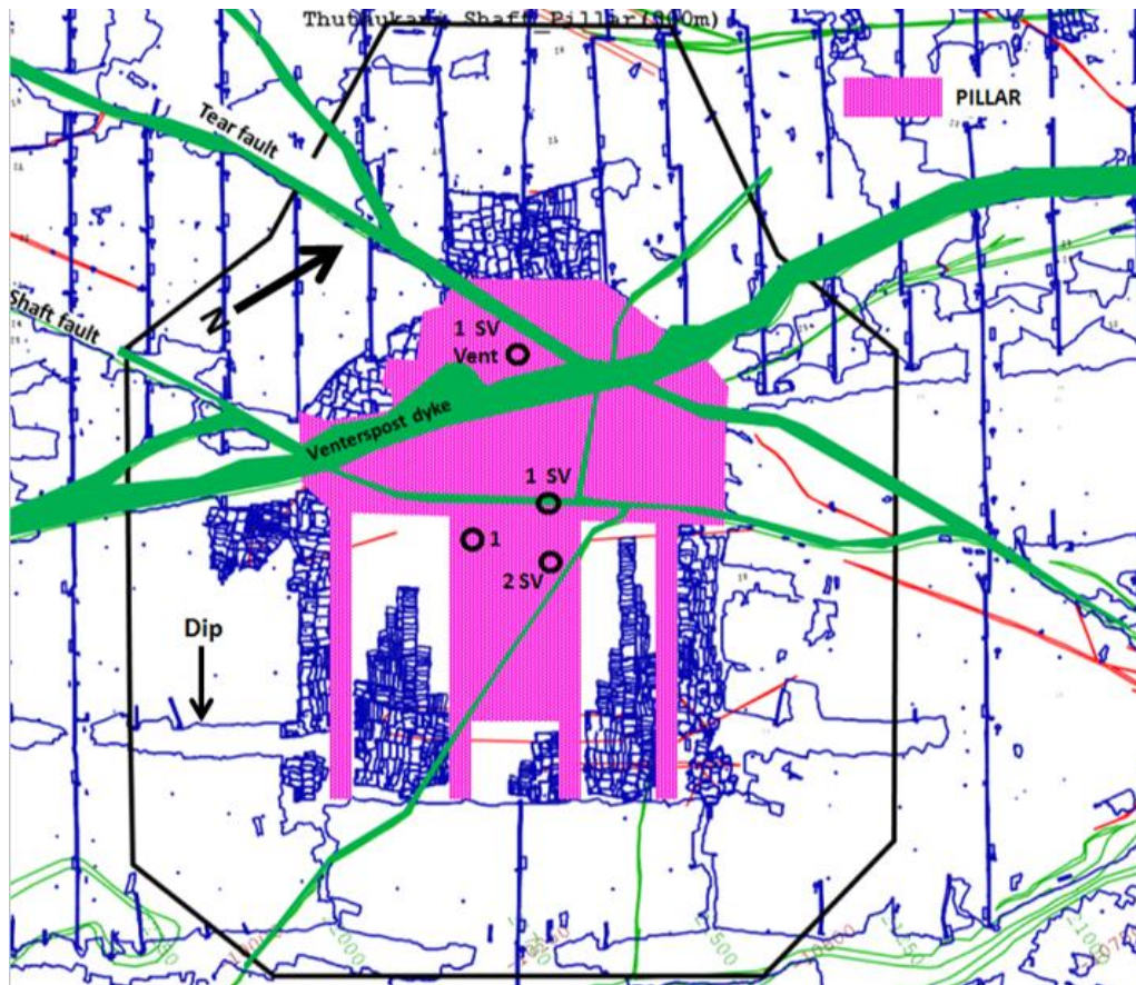
Figure 2: Plan view of the Thuthukani shaft pillar showing the Permanent Pillar, four dip pillars, and the Venterspost Dyke and the Tear and Shaft faults (both containing dyke material). 1 - Main shaft, 1 SV - 1 Sub- vertical shaft, 1 SV Vent - 1 Sub- vertical ventilation shaft, 2 SV - 2 sub-vertical shaft. A black line defines the polygon of analysis
