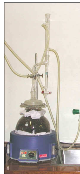
Figure 2.4 Clevenger apparatus used for distillation of plant material.
