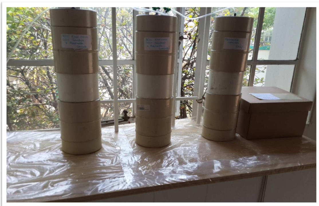
Figure 3 : Long term test rigs post construction. F.l.t.r : Manure : Sawdust 80:20; 80:20; Permeable concrete only
