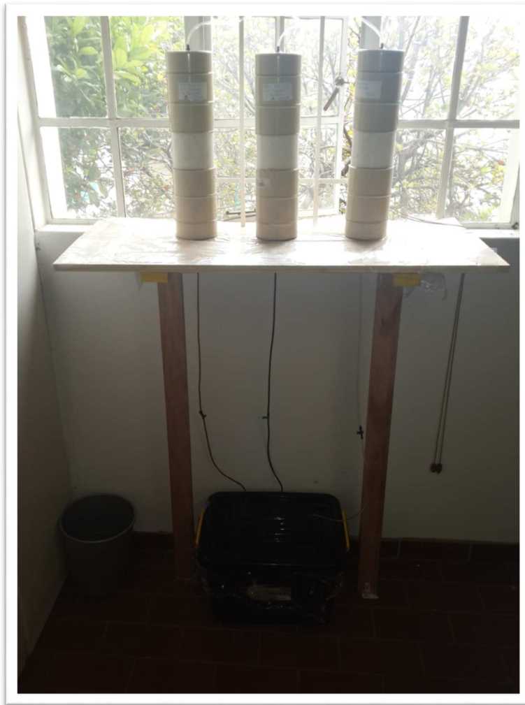
Figure 4: Long term rigs in operation with lined waste bin. F.I.t.r : Manure : Sawdust 80:20; 80:20; Permeable concrete only
