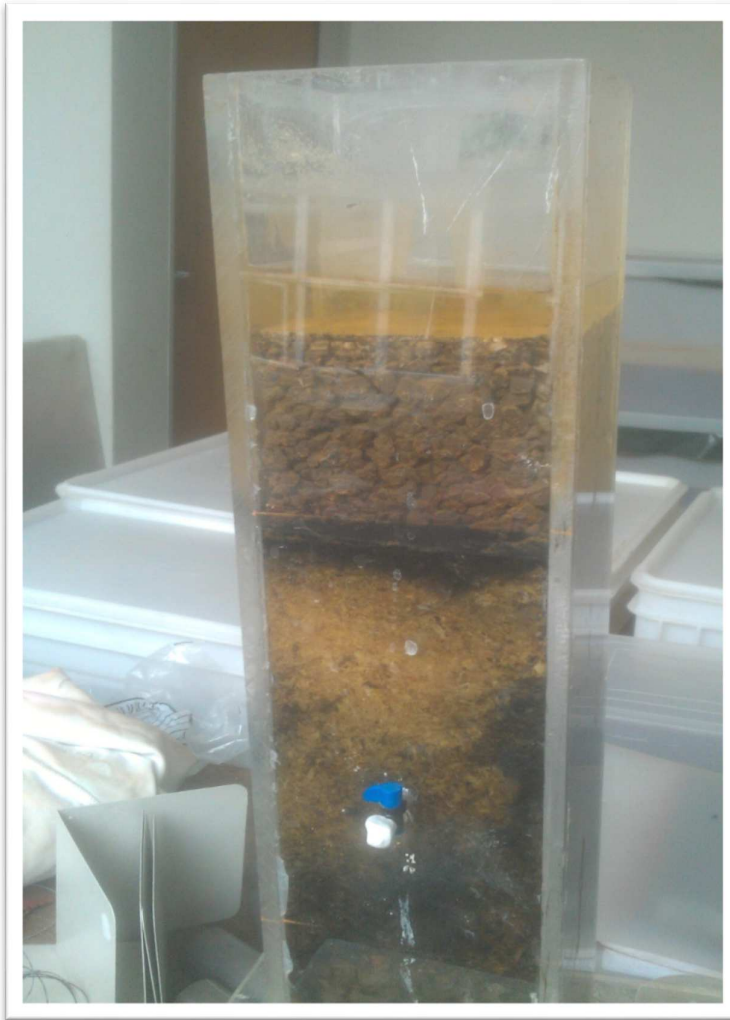
Figure 5: Pilot test rig exhibiting large degree of evaporation. Sawdust 50% and manure 50%
