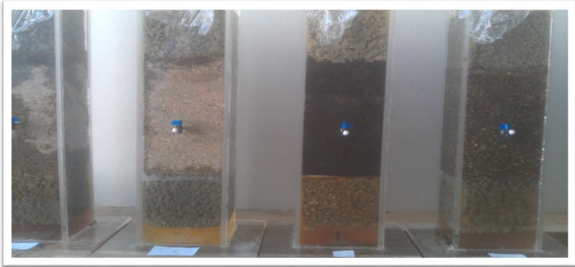
Figure 2: Short term test rigs in operation. F.l.t.r Sawdust : Cow manure: 50:50; 80:20; 0:100; 20:80
