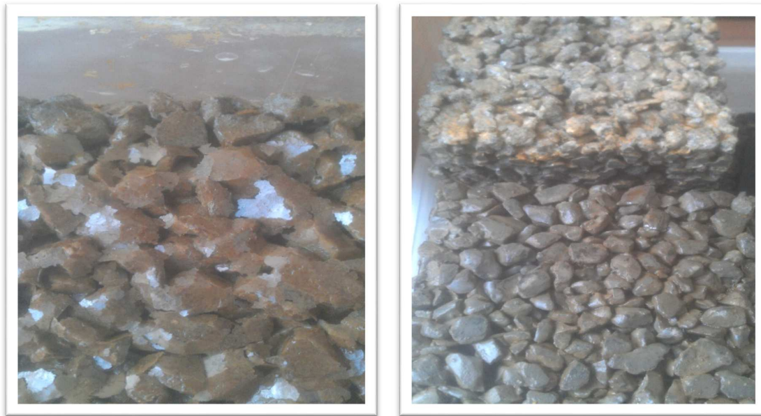
Figure 6 : Precipitate build up on permeable concrete cubes. *The cube on the left experienced exposure to the atmosphere when AMD levels dropped lower than the cubes surface while the cubes on the right remained submerged and show significantly less precipitate. The precipitate is indicated by the brown discoloration
