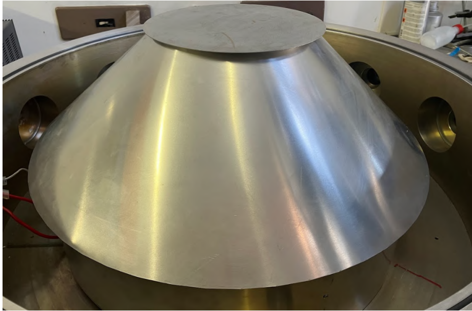
FIGURE 2.2: Total Ion Current Collector
