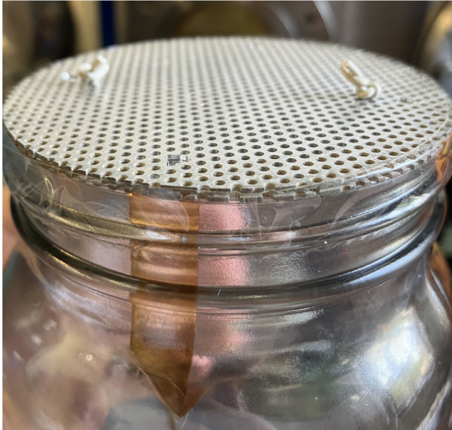
FIGURE 3.8: Final plasma containment vessel with grids attached without lid showing copper tape connection point for screen grid. Note also the grid alignment wires (white).
