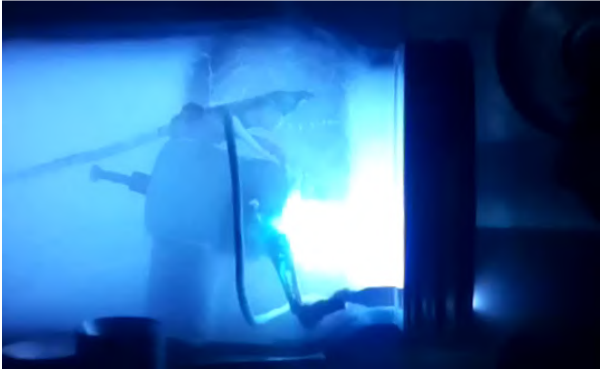
FIGURE 4.6: Typical grid to grid arc.
