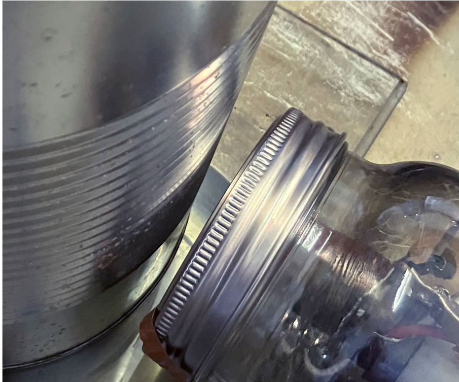
FIGURE 2.5: Tin ion collector. The thruster accel grid is 10mm from the tin. The shape of the tin and the dimpling were expected to reduce secondary electron emission.
