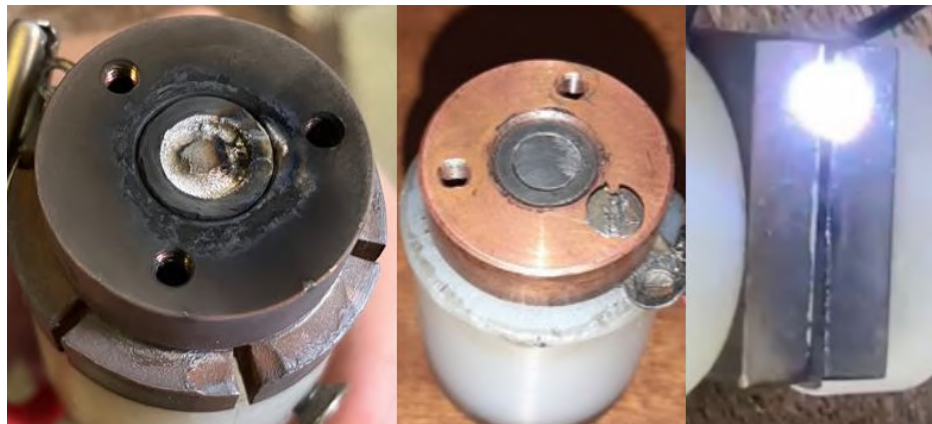
FIGURE 4.1: The three VATs used for the total ion current tests. Left to right: Bismuth coaxial thruster showing clear cathode erosion, coaxial steel thruster with minor erosion and planar steel thruster during arc operation.
