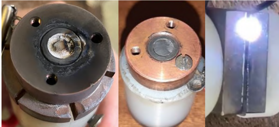
FIGURE 3.2: Left to right: coaxial thruster with bismuth cathode showing erosion, coaxial thruster with steel cathode showing minor erosion, planar steel thruster mid-arc.
