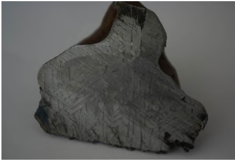
FIGURE 5.1: Acid-etched cut surface of a piece of Sokoto iron meteorite showing relatively coarse Widmanstätten texture. The silver lamellae are kamacite crystals; the darker lines and triangles between them are taenite, schreibersite and/or plessite (intergrowth structure). Base of sample 4.5 cm long. Credit R.L. Gibson
