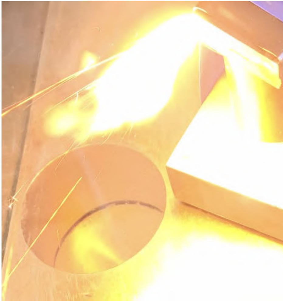
FIGURE A.1: Camera still frame showing planar thruster firing an extended arc pulse of approximately 40ms. The arc color is characteristically blue/purple but in this frame it is clearly seen to be yellow. This frame was taken from the last few ms of the arc pulse, showing clear signs that the glue binding the planar anode and cathode together had suffered an intense heat load and began to melt.
