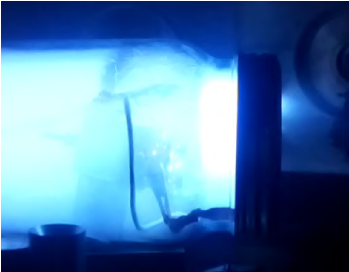
FIGURE 4.5: Typical grid to grid arc.
