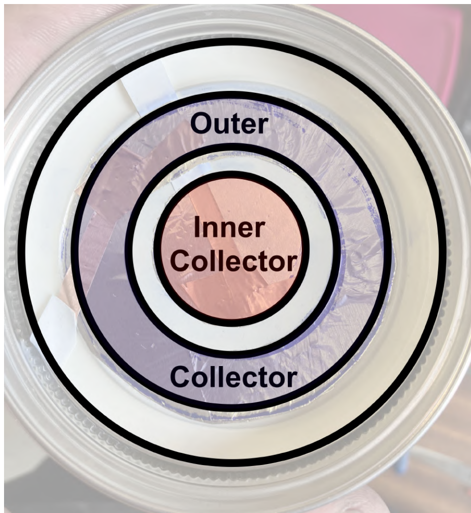
FIGURE 2.6: Annular design ion collector for ion current density measurements.
