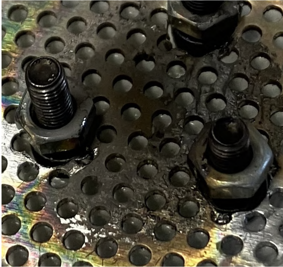
FIGURE 3.5: Extended anode piece removed from VAT. Note the metal deposition and signs of arcing. The grid apertures are 1.5mm diameter.
