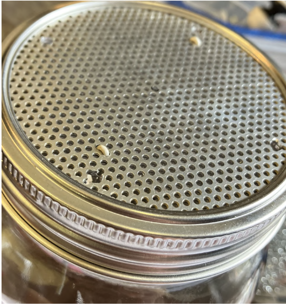
FIGURE 3.7: Design 3: Final upgraded cylindrical plasma containment vessel with grids attached and lid screwed on.
