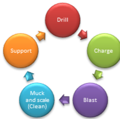
Figure 1.1: The underground conventional drill-and-blast mining cycle (Adapted from Al-Chalabi et al. (2016))
