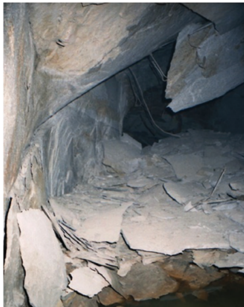
Figure 4.3: Hanging wall collapse in a platinum mine caused by tensile stress (Stacey & Wesseloo 2004)
