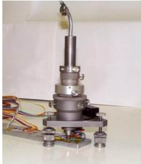
Figure 2.6 Incremental hole-drilling technique instruments use for the determination of residual stresses in carbon fibre reinforced polymer: SINT MTS3000 (left) and Vishay MS200 milling guide (right).
