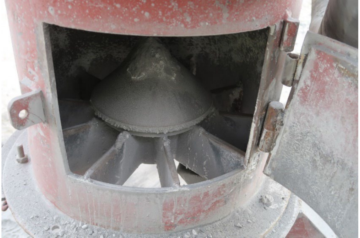
Figure 15: Built-in cone sample splitter in the cyclone.
