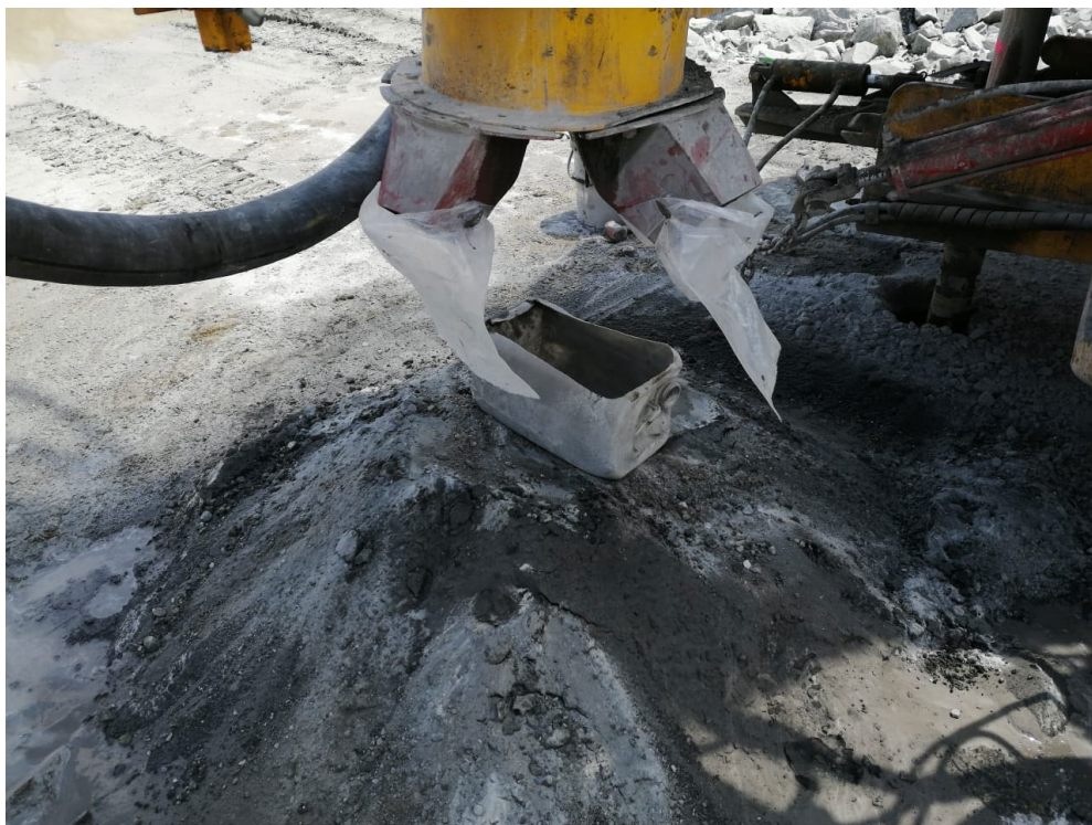
Figure 14: Sample bags tied to the cyclone chutes. The tray is placed underneath the cyclone in the middle to collect the third sample.
