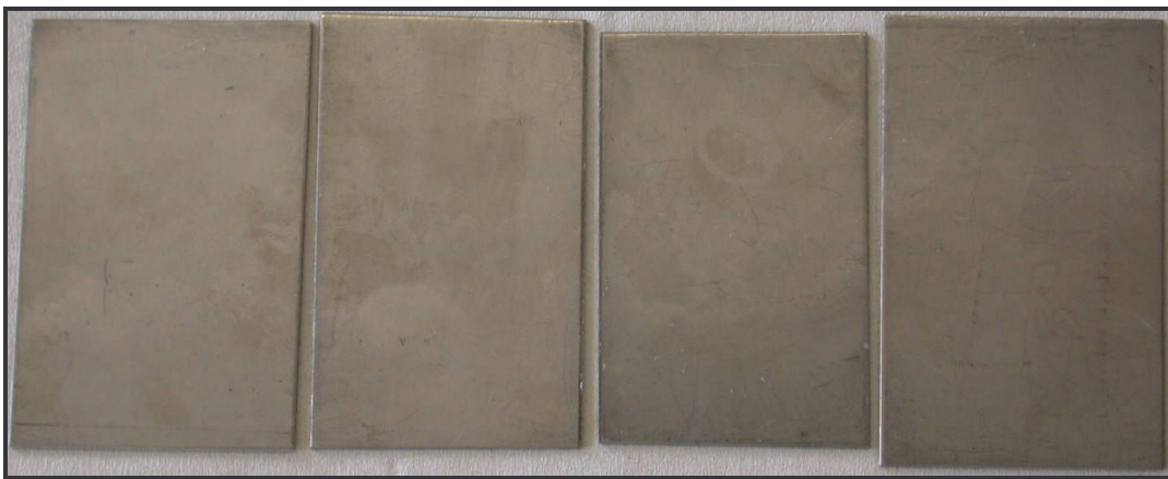
Figure 5.3: Photographs of 304 after total exposure to the petrol condensate, showing little corrosive attack
