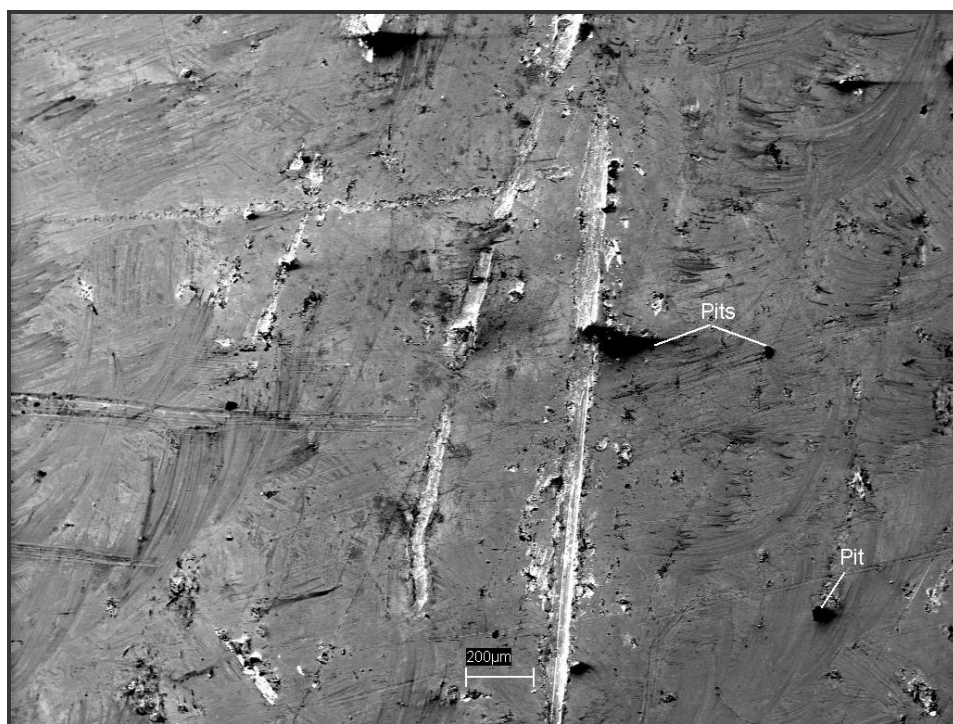
Figure 6.16: SEM micrograph of 434 after total exposure to the modified salt spray test, showing a few pits on a less corroded surface
