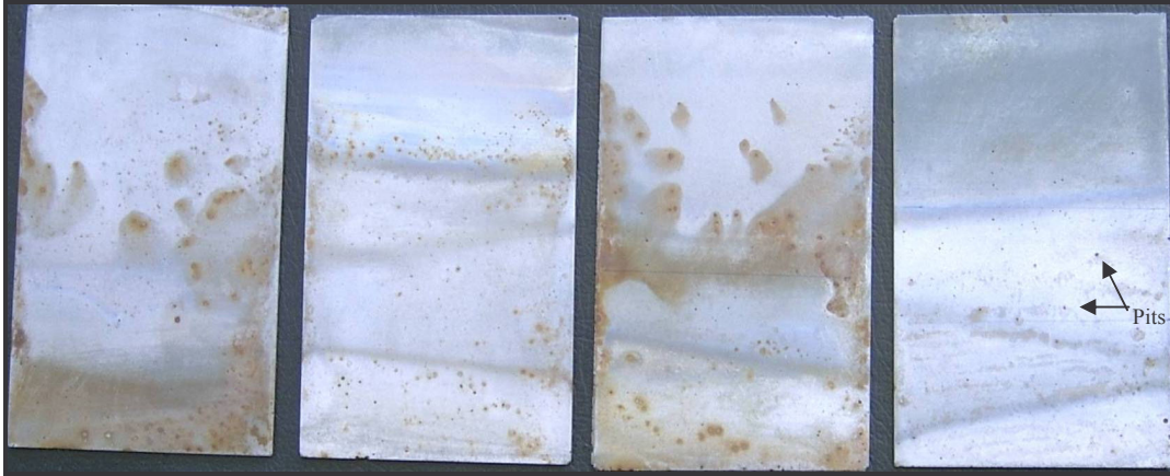
Figure 5.11: Photographs of 409 after total exposure to the diesel condensate, showing pits on the entire surfaces
