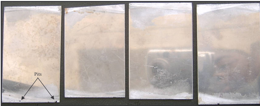
Figure 5.12: Photographs of 434 after total exposure to the diesel condensate, showing corrosive attack and pits at the edges
