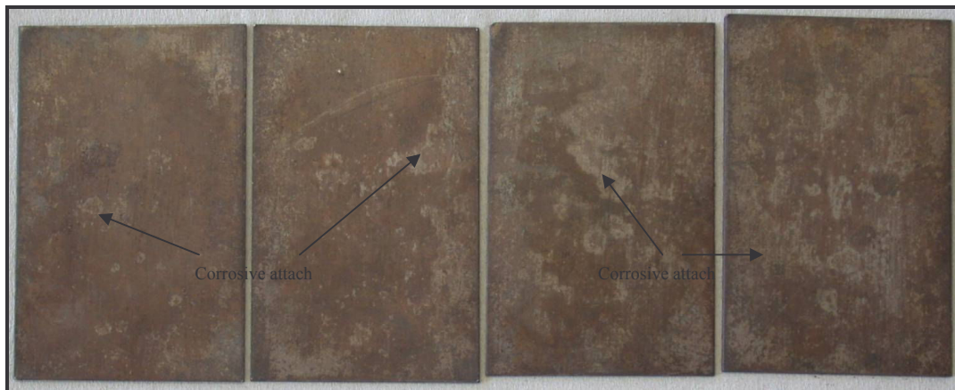
Figure 6.5: Photographs of 409 after exposure to the salt damage test, showing islands of corrosive attack
