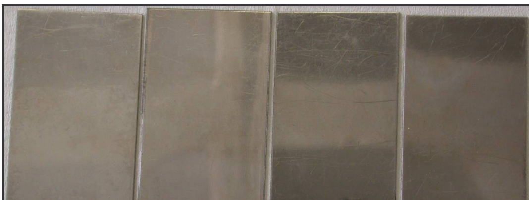
Figure 5.5: Photographs of 434 after total exposure to the petrol condensate, showing little corrosive attack
