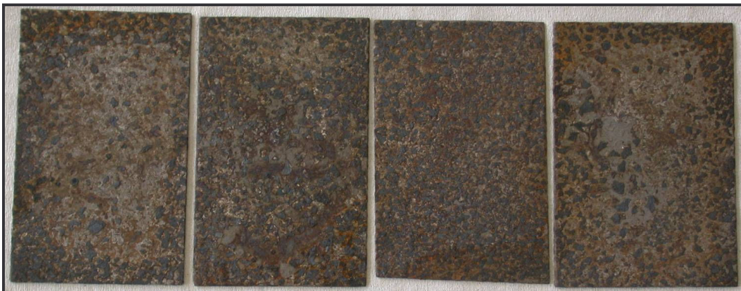
Figure 7.4: Photographs of 304 after exposure to the hot salt test, showing severely corroded surfaces
