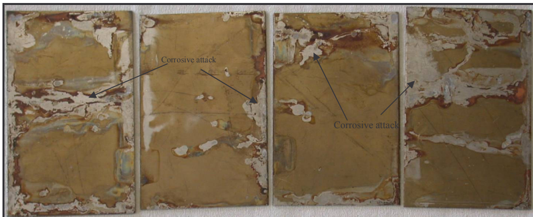
Figure 6.12: Photographs of 409 after exposure to the modified salt spray test (corrosion product removed), showing islands of corrosive attack
