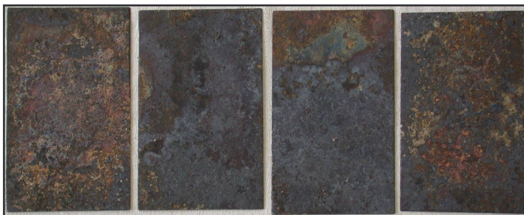
Figure 7.6: Photographs of 434 after exposure to the hot salt test, showing severely corroded surfaces
