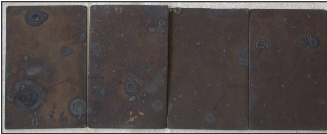
Figure 8.5: Photographs of 1.4509 after exposure to the cyclic oxidation test (after 112 cycles), showing discrete areas of blistering
