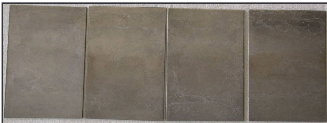
Figure 5.4: Photographs of 409 after total exposure to the petrol condensate, showing little corrosive attack
