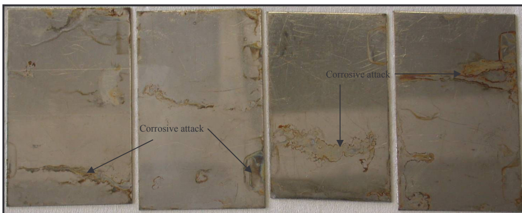
Figure 6.13: Photographs of 434 after exposure to the modified salt spray test (corrosion product removed), showing islands of corrosive attack
