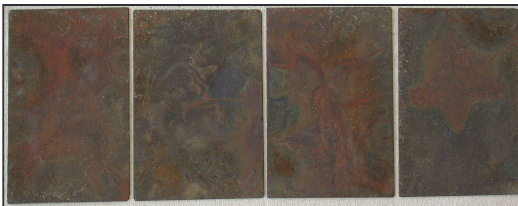
Figure 7.7: Photographs of 1.4509 after exposure to the hot salt test, showing severely corroded surfaces
