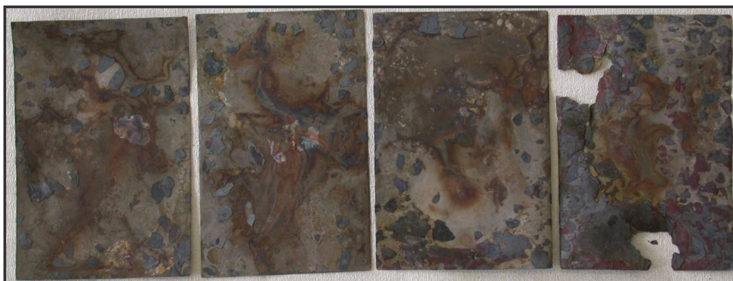
Figure 7.5: Photographs of 321 after exposure to the hot salt test, showing severely corroded and perforated surfaces
