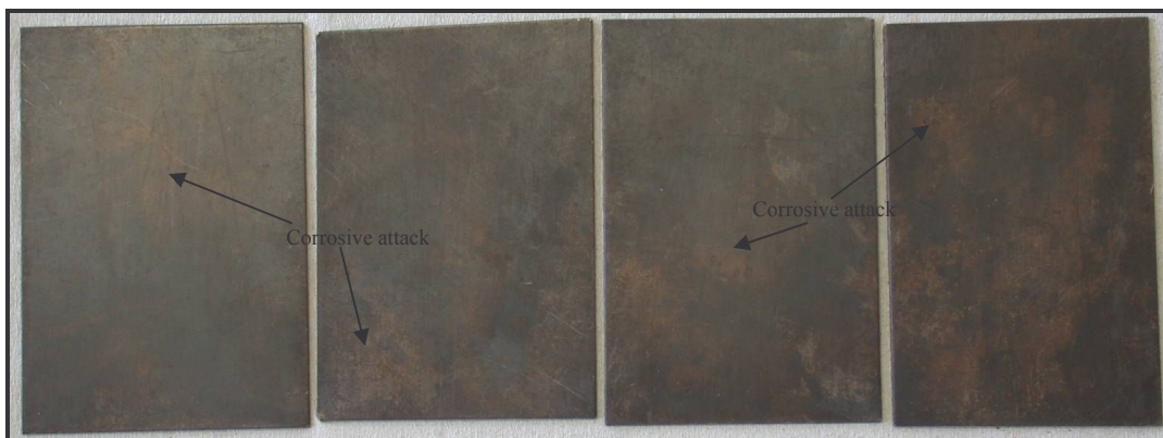
Figure 6.6: Photographs of 434 after exposure to the salt damage test, showing islands of corrosive attack
