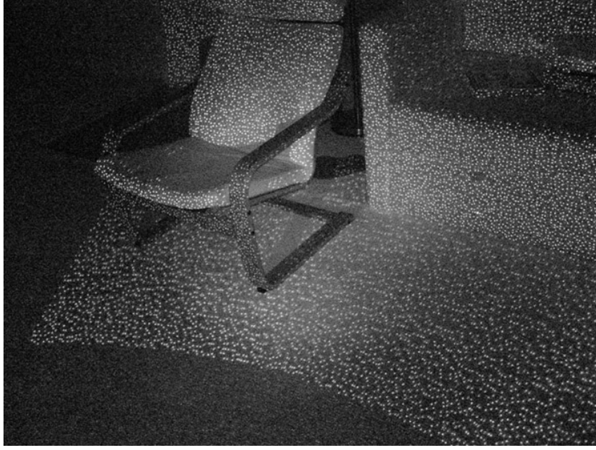
Figure 2.5: The IR pattern used by the Microsoft Kinect [bbzipo, 2017].
