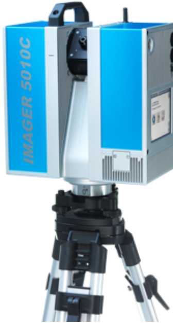
Figure 2.4: The Z+F IMAGER 5010C, 3D Laser scanner [zflaser.com, 2016].
