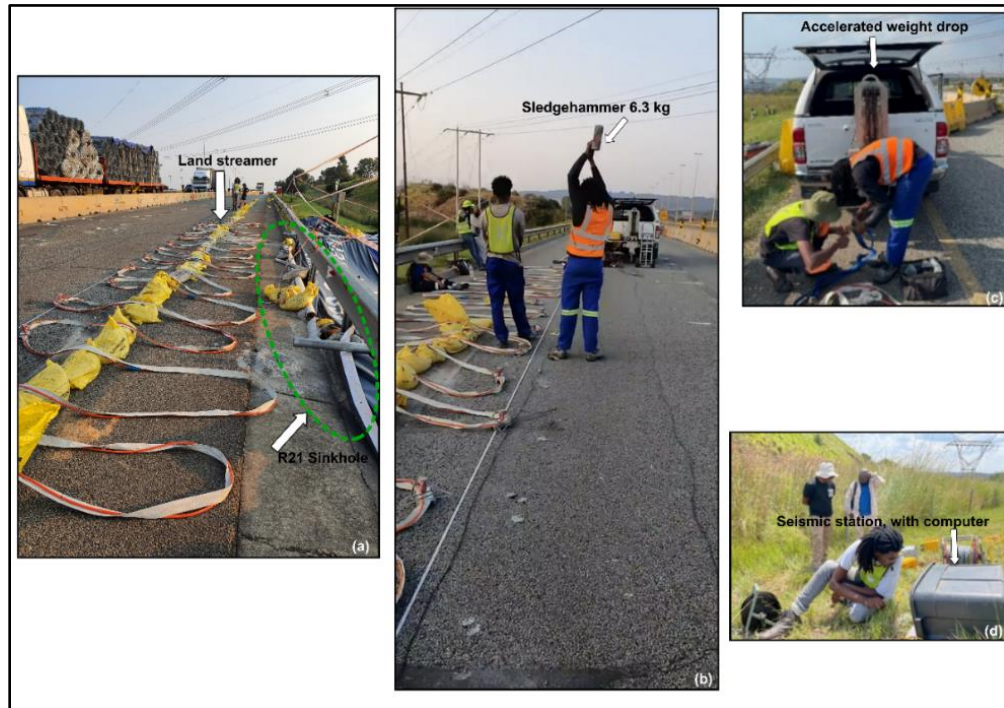
Figure 6.38: Active Multichannel Analysis of Surface Waves data acquisition. (a) Land streamer used for the survey. (b) 6.3 kg sledgehammer used as a source. (c) Accelerated weight-drop mounted at the back for the bakkie. (d) Seismic station.
