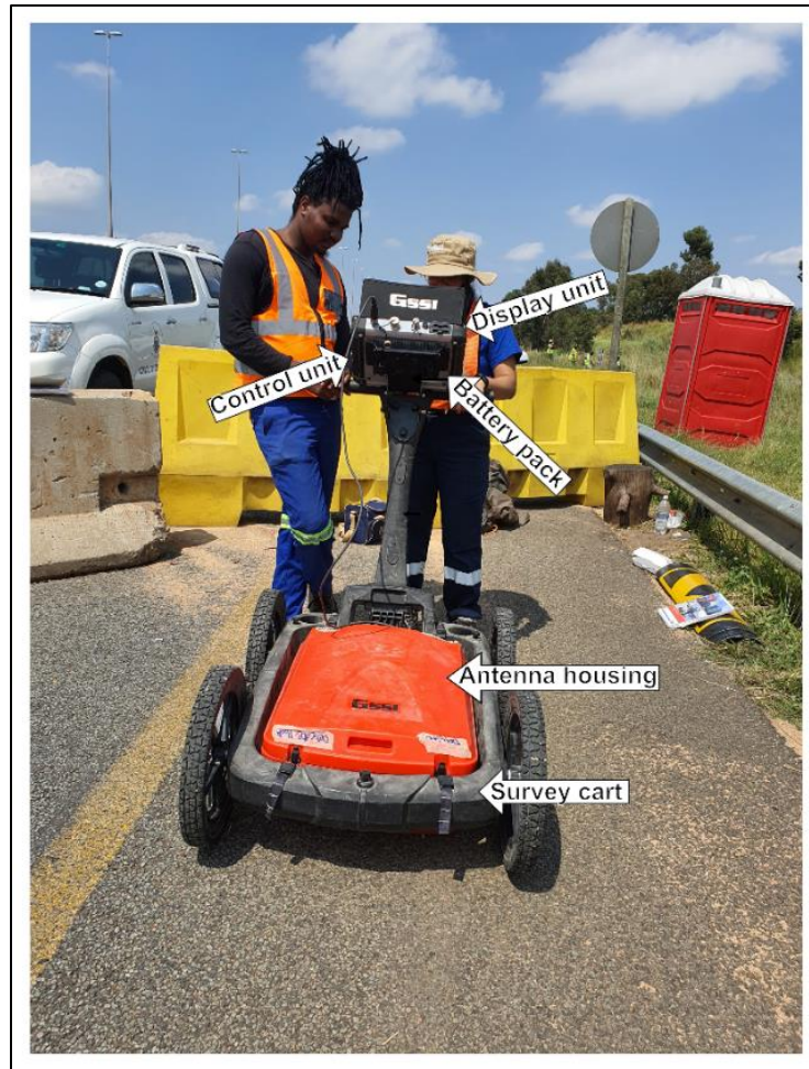
Figure 6.15: GSSI Utility scan PRO SIR 4000 GPR system used in the R21 sinkhole survey.
