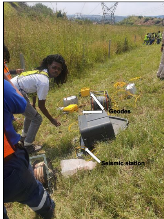
Figure 6.30: Geode seismic data acquisition system.
