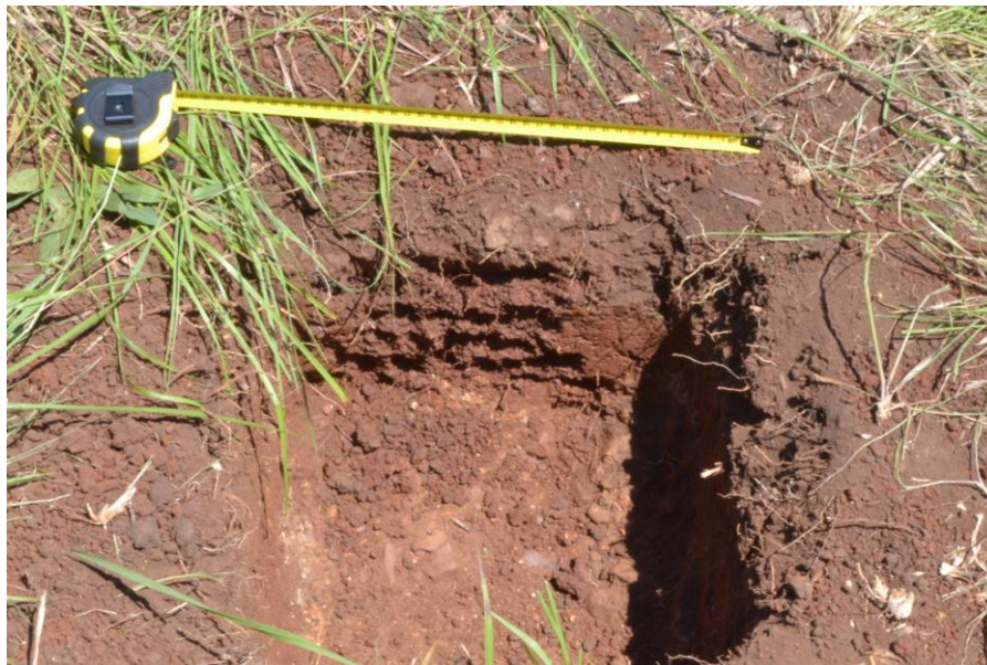
Figure 3.3. Test pit excavated at KG1.
