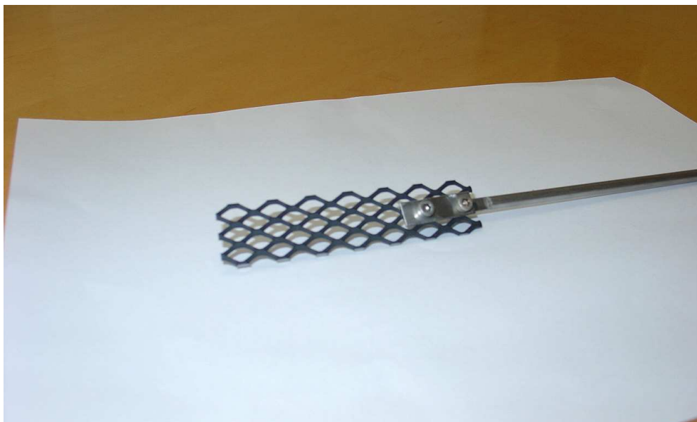
Figure A2 shows a piece of expanded titanium mesh screwed up tight on a rod.
