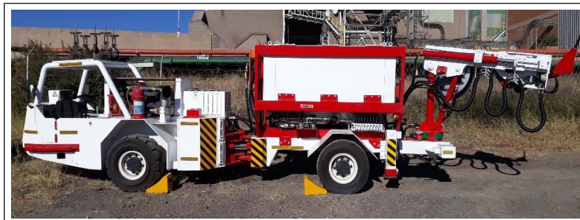
Figure 2.10 AARD-BME long-hole charging rig (Source: On-site picture).
