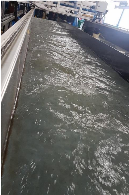
Figure 4-2: 1.0m width flow disturbances (overhead view)
