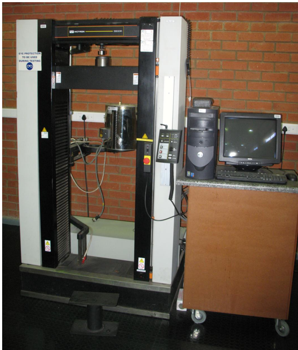
Figure 5.2.1: The 5500R Instron machine in the Element Six laboratory, used for the quasi-static loading test.
