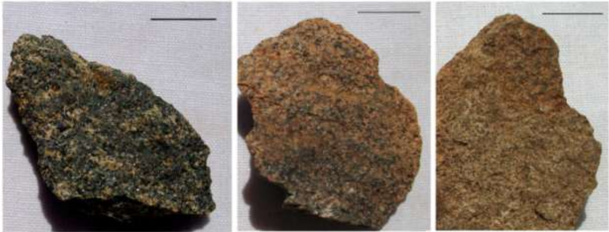
Fig. 3.16: Dolerite from the study area exhibiting various degrees of weathering. Slightly weathered (left) to completely weathered (right). Line is equal to a centimetre.
