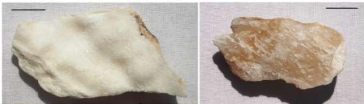
Fig. 3.17: Flowstone from mine workings in the study area. Line is equal to a centimetre.
