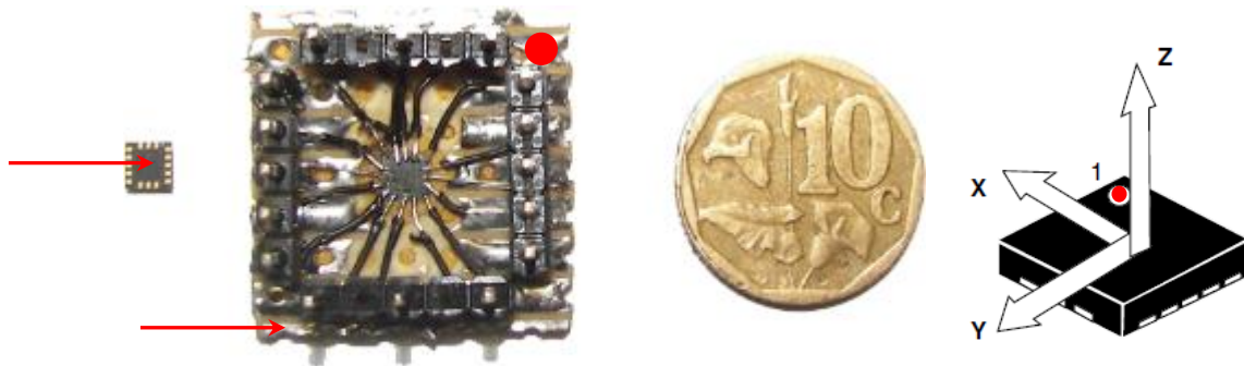
Figure 4.14: LIS3DH mounted using perforated board and comparative sizing with pin mapping
