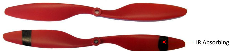
Figure 5.13: IR absorbing marking applied to the blade tips
