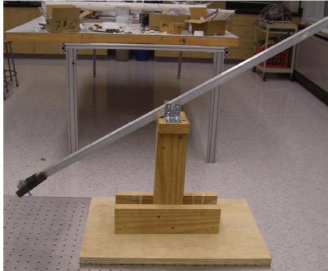
Figure 1.12: Pivot type apparatus set for thrust calculation (DiCesare, et al., 2008)
