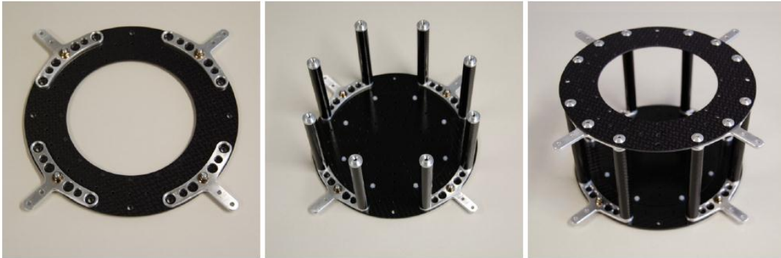
Figure 1.9: A custom built cage for the JAviator (Craciunas, et al., 2008)
