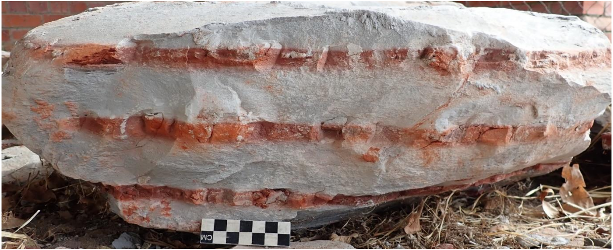
Figure 5.35: Mudstone from Coombs Hill. Stratification in this rock is limited to horizontal alternating red and grey laminae. The red, oxidised layers are discontinuous, and are the product of secondary iron oxidation. They are subordinate in thickness to the grey layers. This stratification is interpreted as evidence for seasonal cyclicity.
