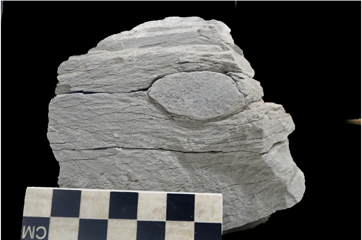
Figure 5.14: A dropstone from Waterloo Farm contained within a block of weathered black shale. Note the slightly tapered margins of the clast, interpreted to be the surface level that the clast occupied after impact where the margins subsided slightly. Above this level shale laminae onlap the clast.
