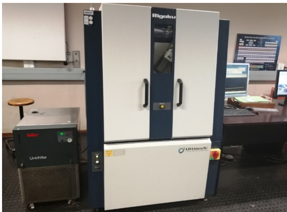
Figure 3.2: Photograph of what an XRD machine looks like. A Rigaku Ultima IV machine was used to do the clinoptilolite analysis
