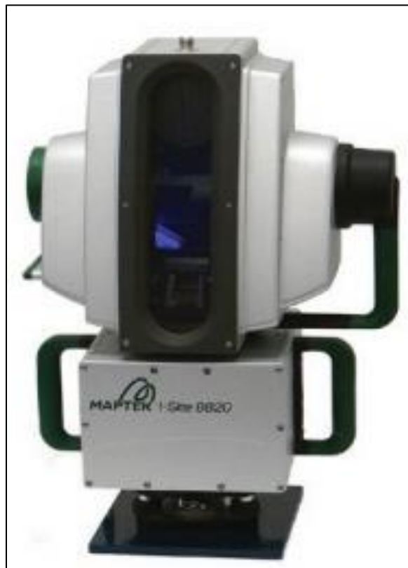
Figure 9: The Maptek I-Site 8820 Laser Scanner
