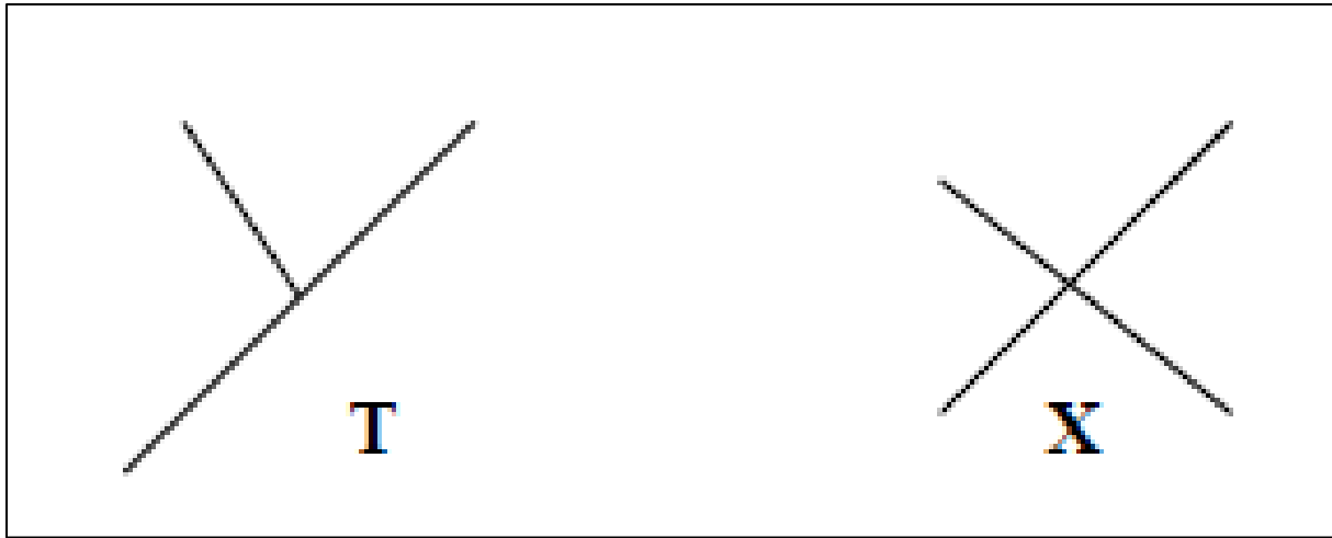
Figure 5: T-type and X-type termination (adapted from Elmo, et al. 2014)
