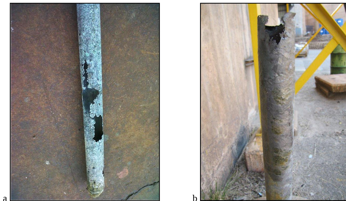
Figure 2.4: (a) Corrosion in the liquid phase, and (b) in the vapour phase above HF liquid level of Monel dip tubes installed on March 2012 into Storage tanks V1460 and removed 2 weeks later due to excessive corrosion (Valkenburgh, 2012e).
