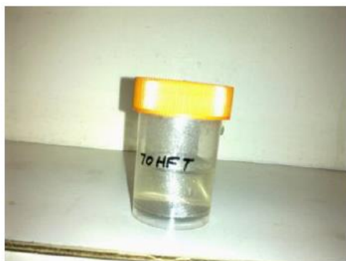
Figure 2.8: (a) 70% technical grade HF indicating no visual reaction with iron powder, and (b) 70% industrial HF showing some visible reaction had occurred with the iron powder (Valkenburgh, 2012c).
