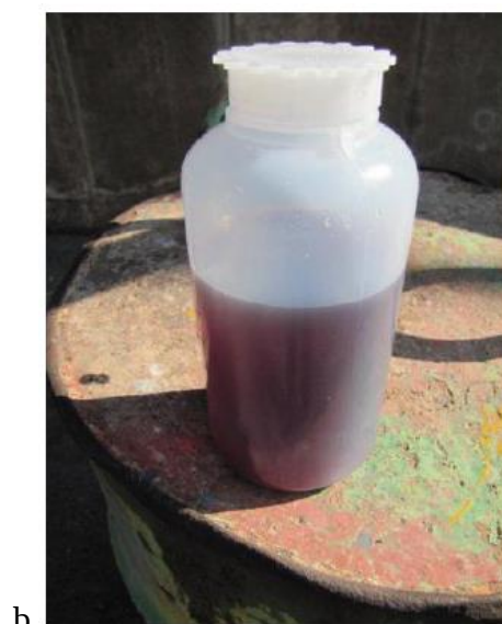
Figure 2.6: (a) \text{H}_2\text{SO}_4 as-received from the supplier's tanker, and (b) \text{H}_2\text{SO}_4 from the bottom of the plant storage tanks where the impurity which settled out was predominantly \text{FeSO}_4 (Valkenburgh, 2012c).
