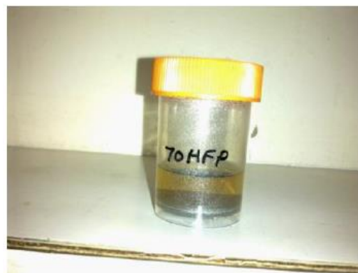
Figure 2.8: (a) 70% technical grade HF indicating no visual reaction with iron powder, and (b) 70% industrial HF showing some visible reaction had occurred with the iron powder (Valkenburgh, 2012c).
