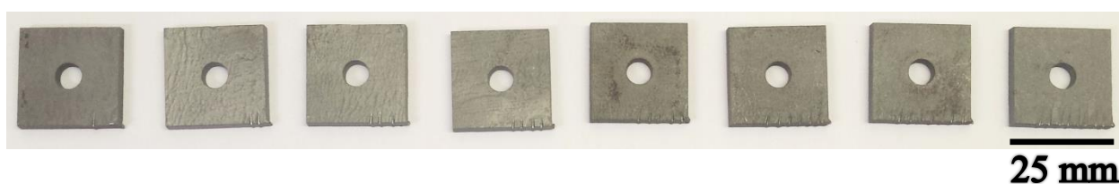
Figure 4.4: Examples of final coupons, after washing with acetone, prepared for corrosion immersion tests, with sequencing marks on the bottom edges.
