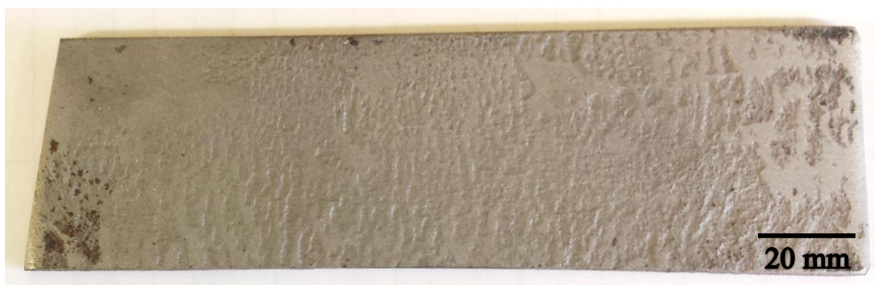
Figure 4.2: Example of the original steel received from hot rolling received after sand-blasting.
