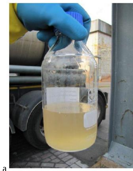
Figure 2.6: (a) \text{H}_2\text{SO}_4 as-received from the supplier's tanker, and (b) \text{H}_2\text{SO}_4 from the bottom of the plant storage tanks where the impurity which settled out was predominantly \text{FeSO}_4 (Valkenburgh, 2012c).
