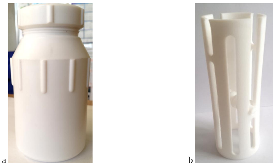
Figure 4.7: Corrosion reactor components: (a) Teflon bottle, and (b) cylindrical corrosion rack with Teflon rod to the suspend coupon.
