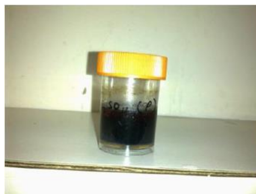
Figure 2.7: (a) 98% Laboratory grade \text{H}_2\text{SO}_4 indicating no reaction with iron powder, and (b) \text{H}_2\text{SO}_4 from the supplier which had reacted to form a thick brown residue with the iron powder (Valkenburgh, 2012c).
