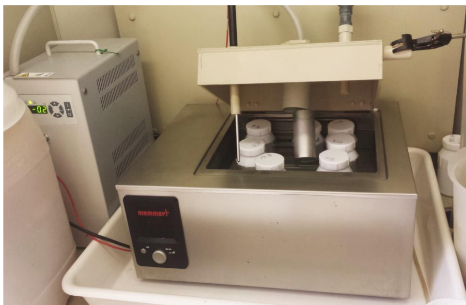
Figure 4.6: Water bath with immersion cooler set-up for corrosion tests.
