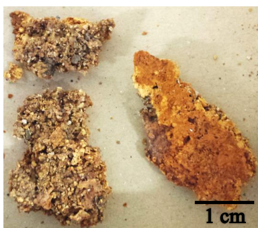
Figure 3.6: Removable scale, collected from below the liquid band (point 5 in Figure 3.4) on the inside of the HF storage vessel (Figure 3.2b), for XRD analysis.
