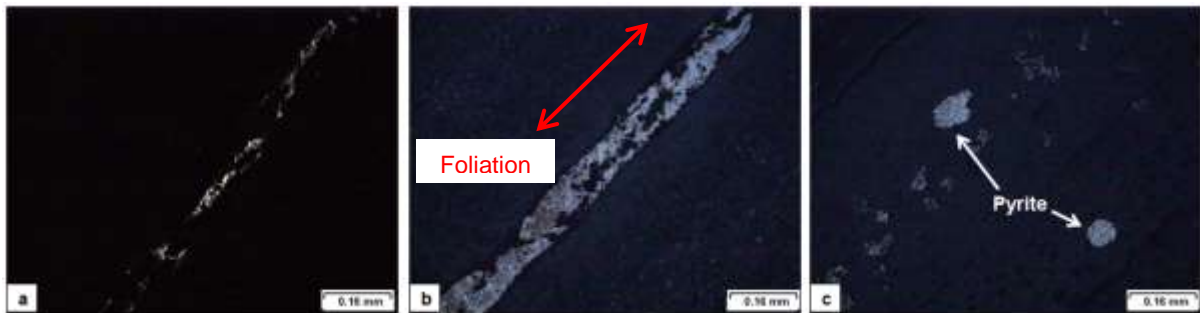
Figure 6.96: Thin section results for the carbonaceous shale sample (sample W41).
