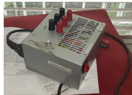
Figure D-1: ATX power supply for strain gauge measurement system
