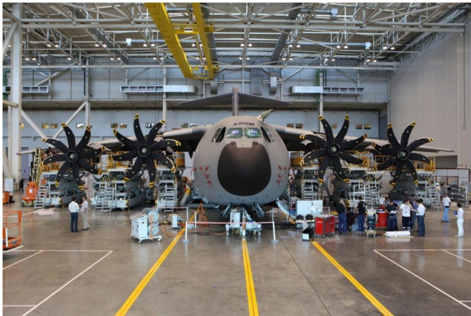
Figure 2-5: Image of propeller size on A400M and blade number
