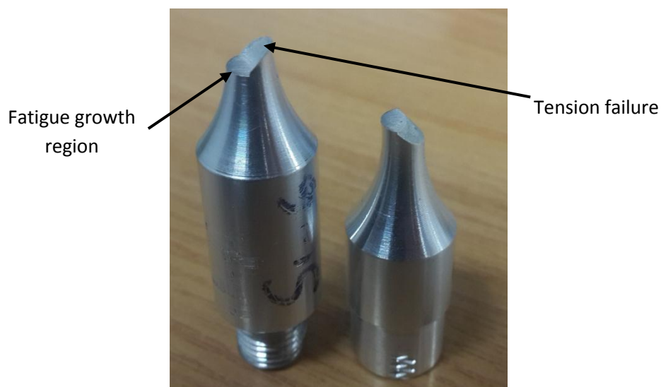
Figure 5-5: Failed specimen showing tension failure (H1-S1-6)
