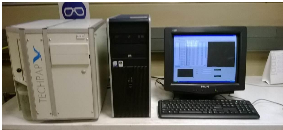
Figure 3.5: TECHPAP Instrument to measure MFWT
