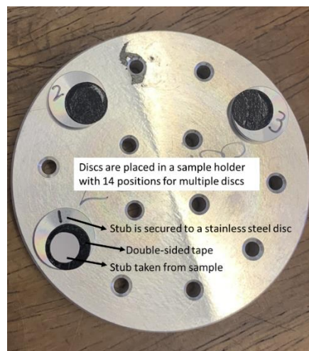
Figure 4: Stub secured to disc that is placed on sample stage
