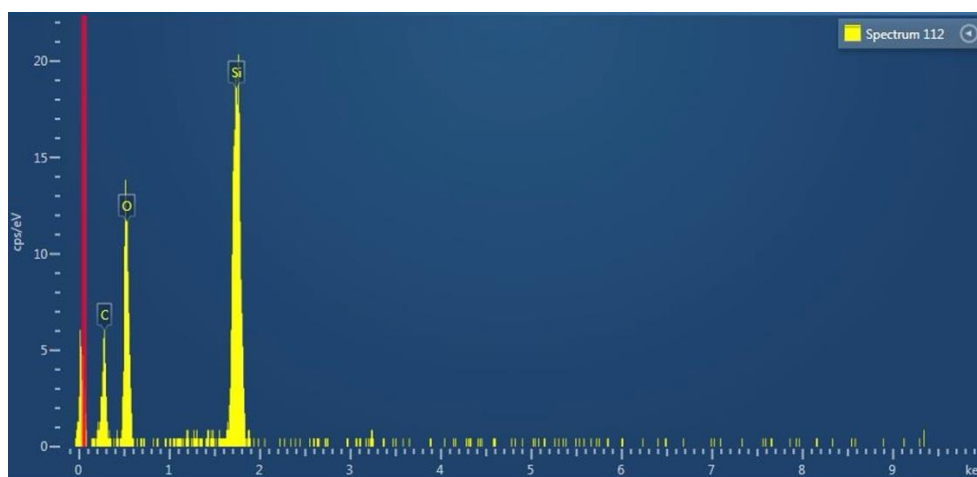
Figure 12: EDS confirms the presence of \text{SiO}_2 dust with the carbon coating to improve conductivity
