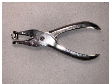
Figure 3.3: Punch that was used to remove a specimen from the sample
