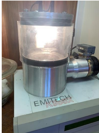
Figure 7: Coating of samples using carbon evaporation
