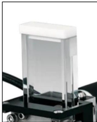
Figure 13: Fraction cell of the LLS instrument
