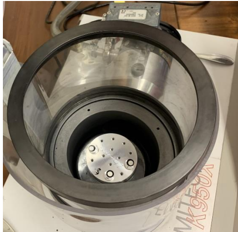
Figure 5: Stubs on sample stage placed inside the carbon evaporator
