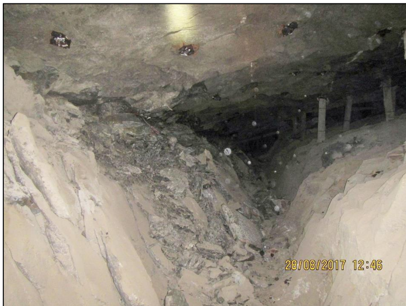
Figure 38: Lateral dilation of the Merensky Reef pillar into the ASG
