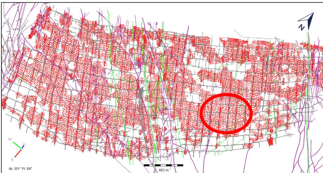
Figure 5: The Merensky Reef extraction at Tumela 1 Shaft. The circled area is where the highest rate of seismicity is occurring at Tumela 1 Shaft. The white areas indicate unmined areas (areas that will still be mined such as potholes)
