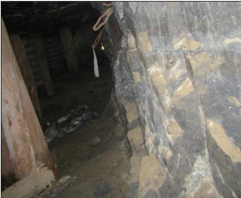
Figure 14: The superimposed UG2 Reef pillar corner, at the panel below the 11-32W Merensky Reef dynamic pillar failure, which had little sign of damage
