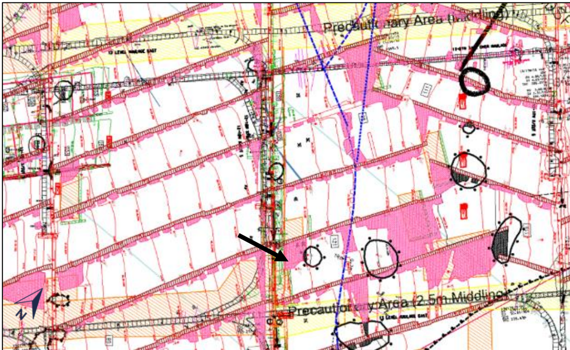
Figure 45: Plan showing the 13-18W UG2 Reef (green) and Merensky Reef stopes (red). The pink hatched areas were the Merensky Reef pillars. The black arrow indicates the pillar of interest. This area has not been understoped by UG2 Reef mining
