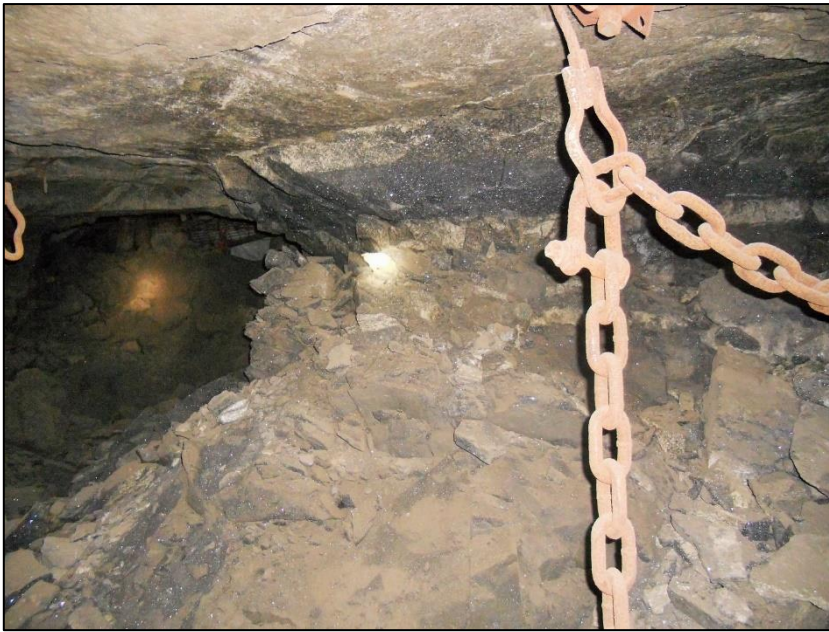
Figure 44: The failed UG2 Reef in-stope pillar
