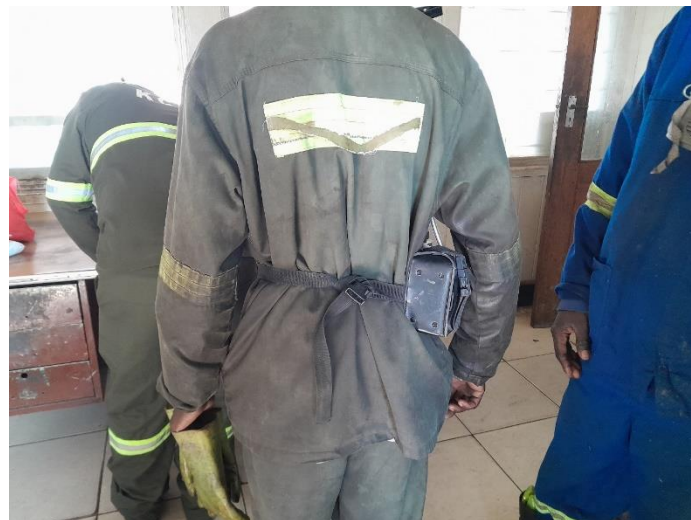
Figure 2.3 Illustration of air sample collection pump on worker's waist
