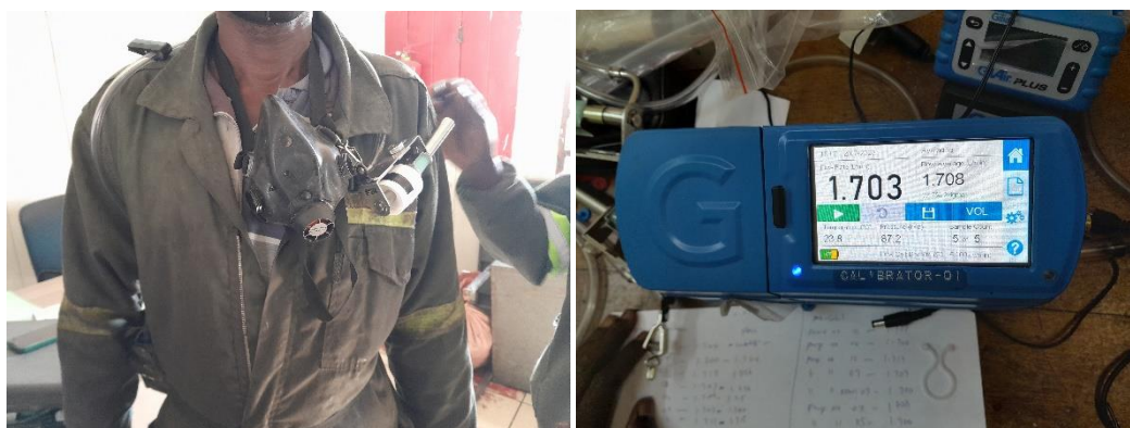
Figure 2.4 Lead air-sampling setup in the work environment
