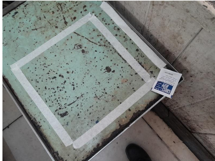
Figure 2.5 Lead surface sampling with SKC lead dust wipes over 30 cm x 30 cm area
