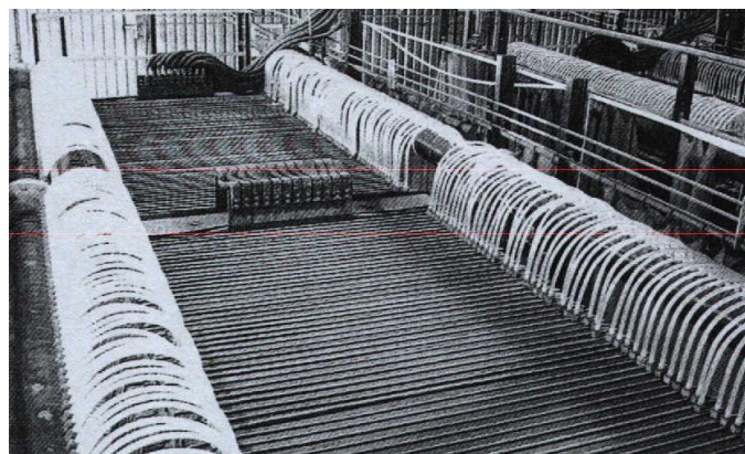
Figure 2: A bank of cells in series for electrolysis of brine at NCP Chloorkop
