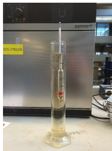
Measuring solution density
