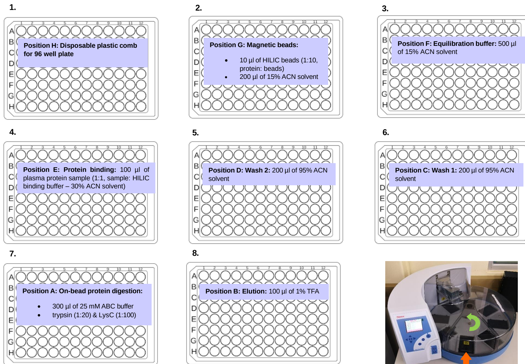
Figure 2.3: Diagram of 96-well plate positioning in KingFisher Flex™ for sample clean-up and on-bead protein digestion. Eight 96 deep-well plates shown are labelled 1-8, in order of plate loading sequence as per the in KingFisher Flex™ system prompting.
