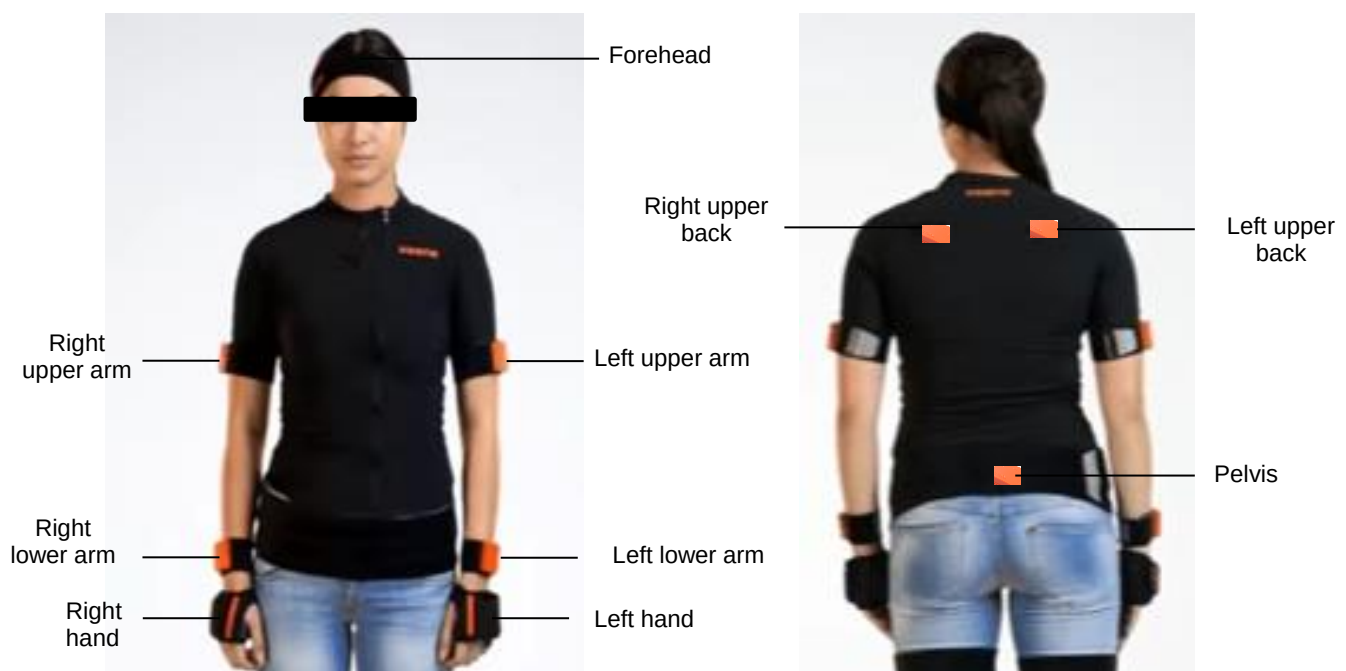
Figure 5.1: MVN BIOMECH® ® inertial motion sensors set up
