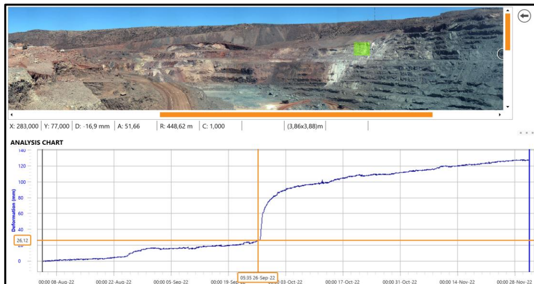
Figure 4-2. Slope stability radar deformation data for Event1.
