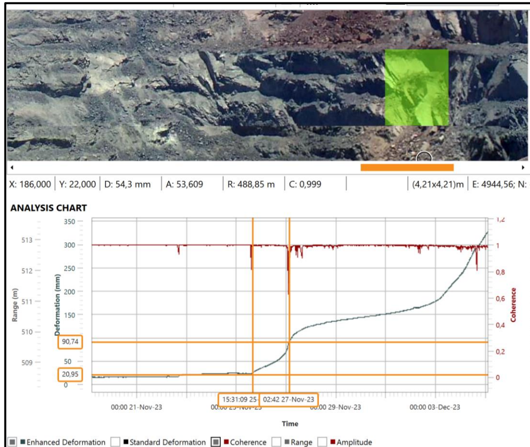
Figure 3-9. Typical deformation data (in millimetre) extracted from the slope monitoring database (GroundProbe).
