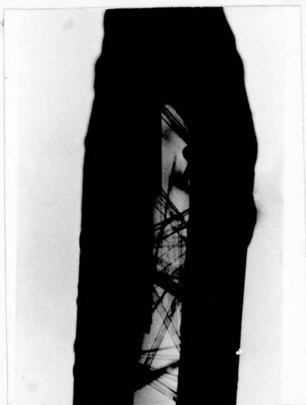
Lath-like crystals of \text{Mg}_4\text{Al}_2\text{Ti}_9\text{O}_{25}
