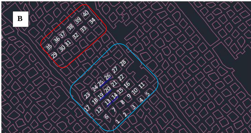
Figure 4.2-1- Panel where coaling has previously taken place and the pillar analysed, where (a)- coaling panel chosen and (b) the pillars chosen for the investigation (AngloAmerican (Thermal coal), 2017)
