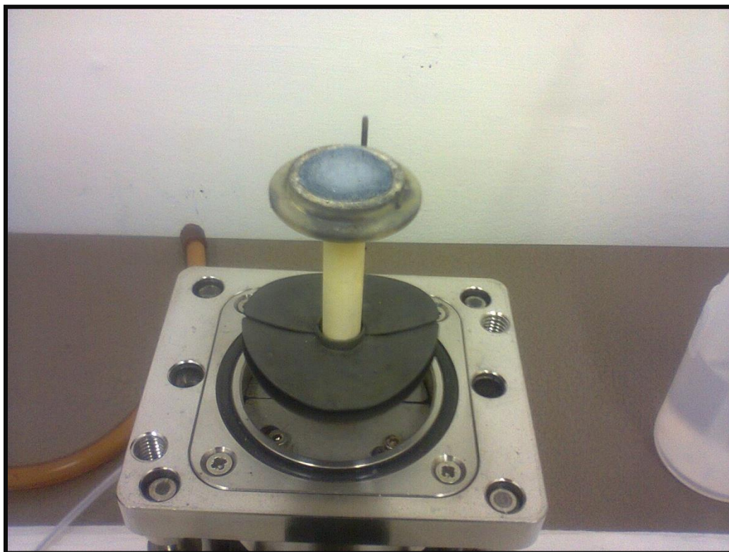
Figure 4.10: Bruker D8 Advance sample holder with the product after the COXA analysis showing the dark blue product.
